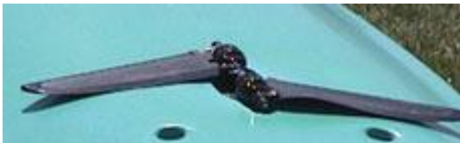
FIGURE 8: MIRAGE DRIVE SYSTEM FLAT AGAINST HULL
