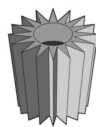
Unlike the first design, a Peltier cooler would be attached directly to the inside of a large piece of metal with maximized surface area (left). The cold metal would condense water out of the air which would then drip down, pass through a charcoal filter and be collected into a large storage container.
