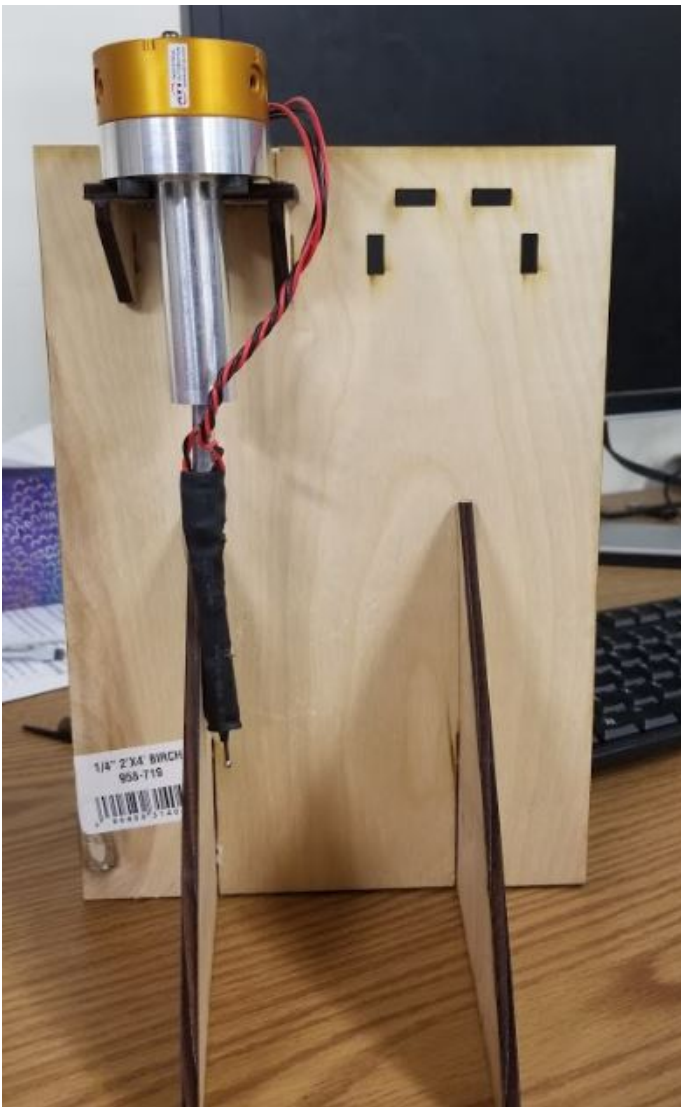
Fig. 21. Prototype tool holder with EOAT stored
