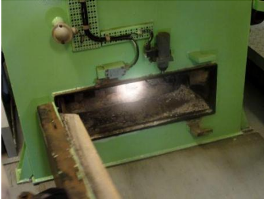
Figure 9: Incinerator used for burning sludge
