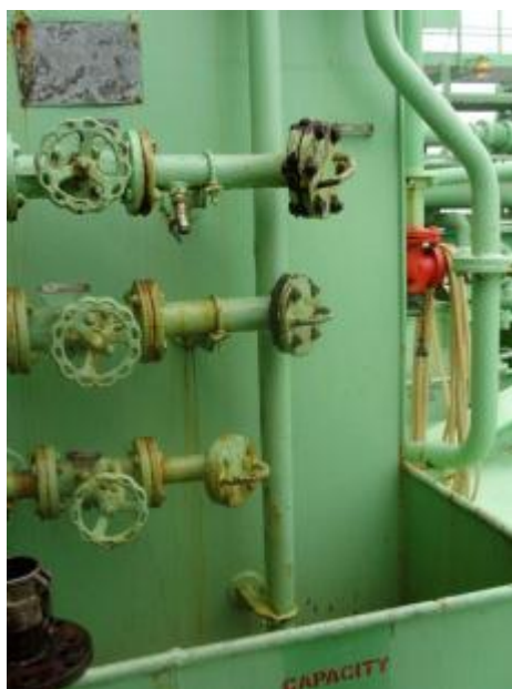
Figure 64: The hookups to pump sludge off of the vessel.
