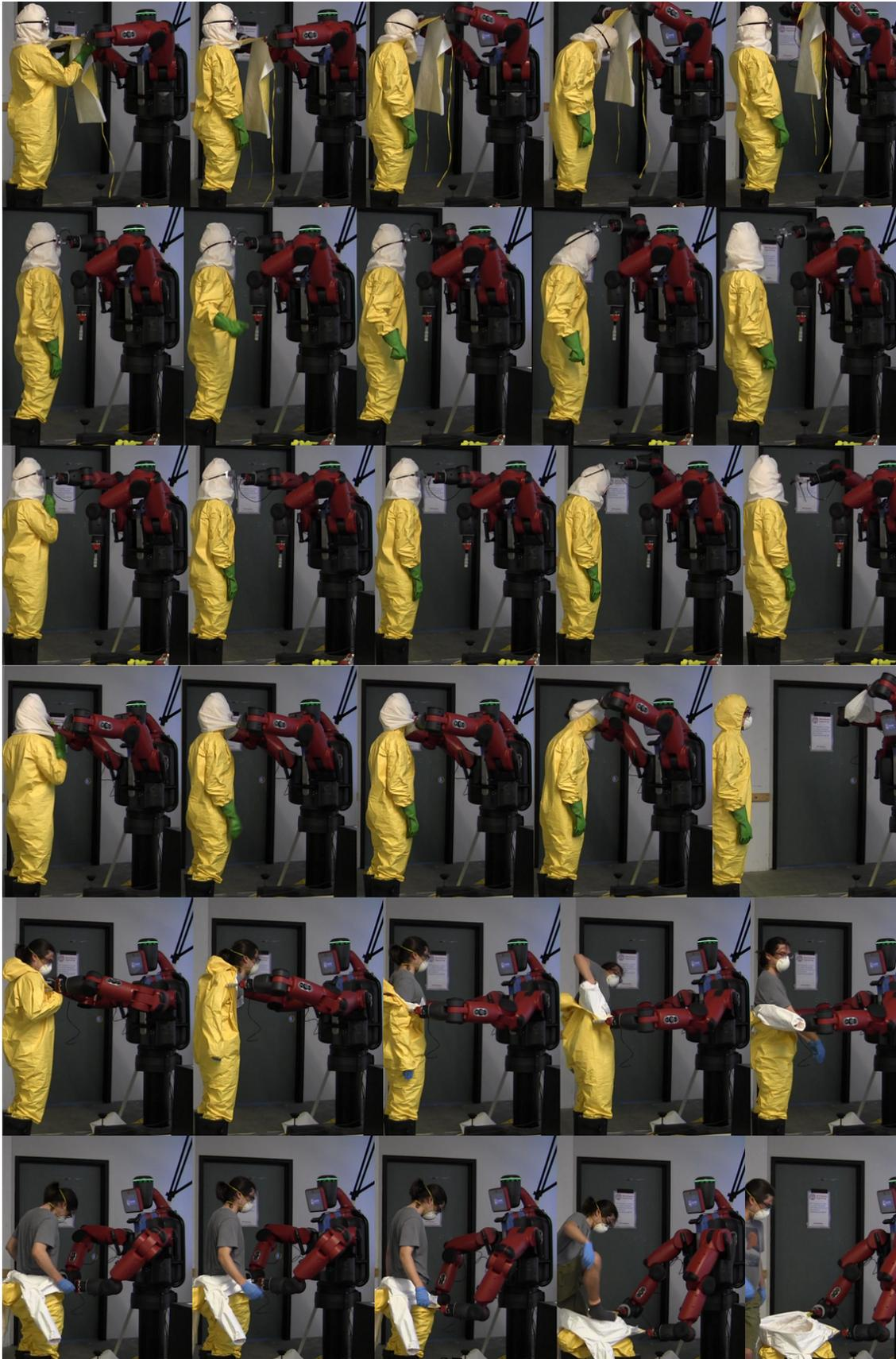
Figure 7.1: Robot-Assisted doffing using transfer motions.
