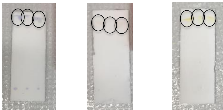
Figure 10. MOF based TLC plates with (from left to right) crystal violet run in 9% methanol in DCM, diacetyl ferrocene in 3% methanol in DCM, and ferrocene in pure hexanes.
