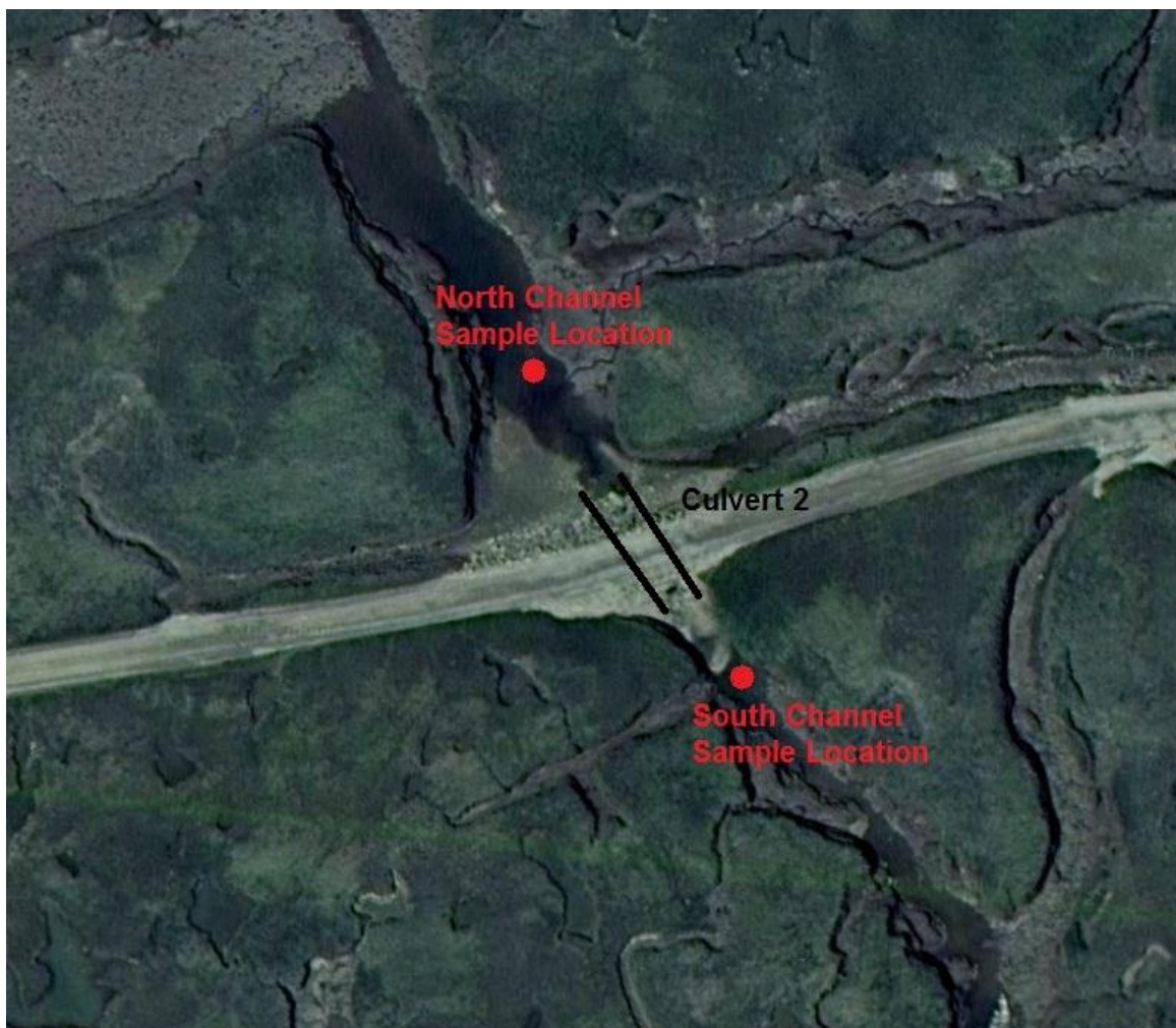
Figure 15: Sample Locations for Deployment of Depth Probes at Culvert 2
