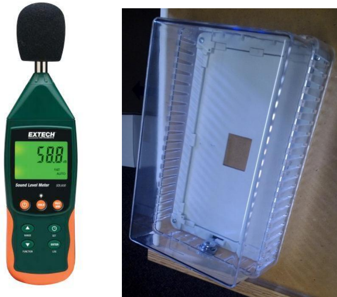
Figure 3: Extech SDL-600 Sound Level Instruments (left) and Sensor Housing (right)
