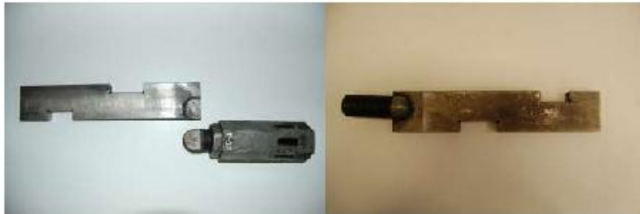
Broken Short Key
