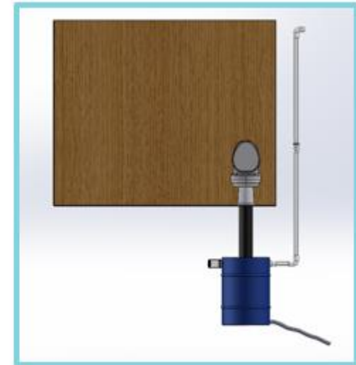
[A representation of a composting toilet system]
