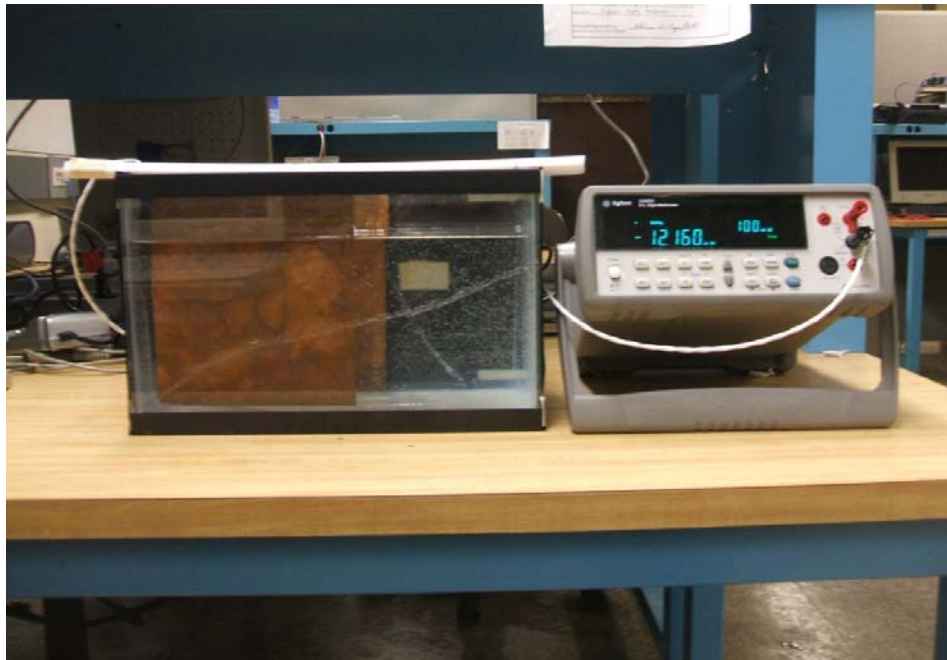
Figure 8: Our initial setup consisting of two copper plates immersed in NaCl solution inside a glass tank.
