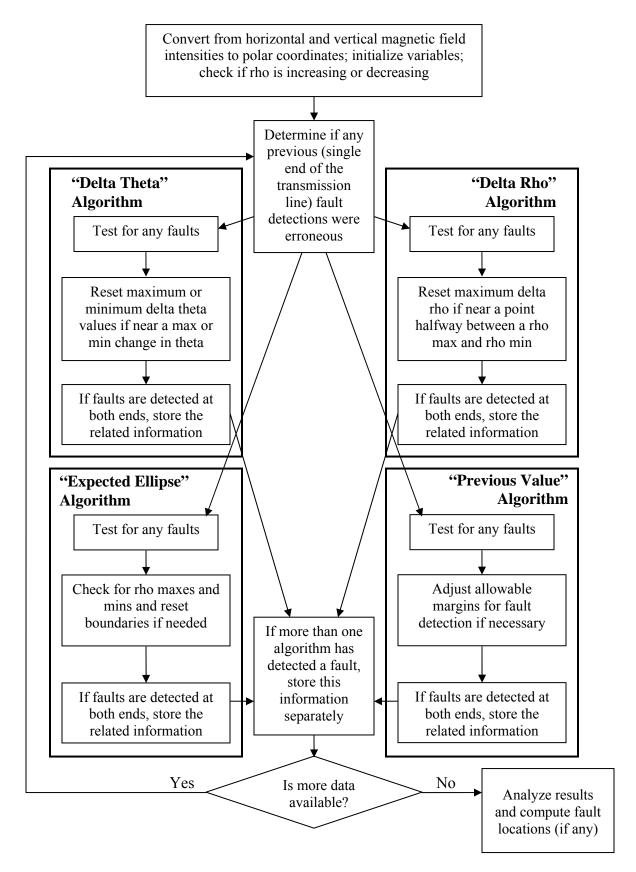
**Figure 4-16 – Fault Detection Algorithm**
