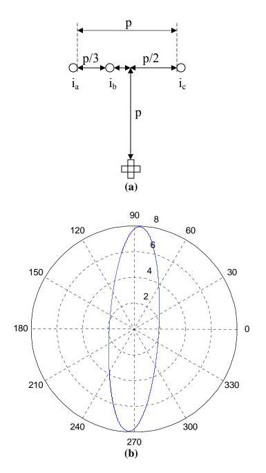
Figure 3-2 – Elliptical rotating magnetic field produced by three-phase, three-conductor system (a) – Conductor geometry; (b) – Magnetic field for p=2m
