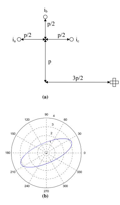
Figure 3-12 – Delta conductor configuration and magnetic field with sensors shifted significantly (a) – Conductor geometry; (b) – Magnetic field for balanced currents, p=2m
