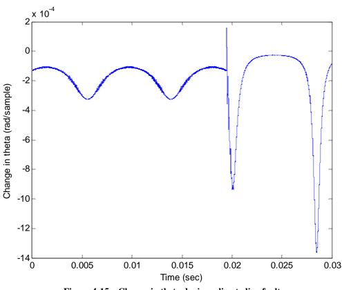
Figure 4-15 – Change in theta during a line to line fault
