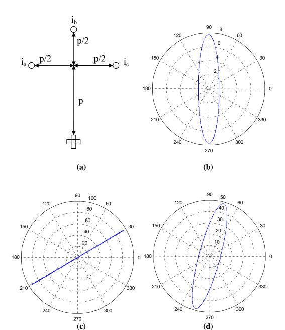
Figure 3-5 – A delta conductor configuration and plots of its magnetic field (a) – Conductor geometry; (b) – Magnetic field for balanced currents, p=2m; (c) – Magnetic field for a line to ground fault on phase a, p=2m; (d) – Magnetic field for line to line fault on phases a and b, p=2m
