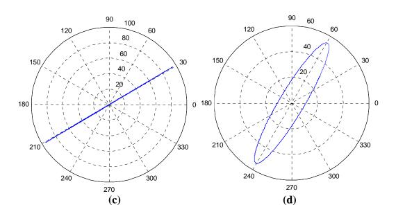
Figure 3-6 – A different delta conductor configuration and plots of its magnetic field
