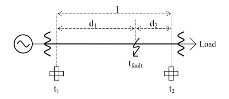
Figure 3-13 – Distances and times used in fault location
