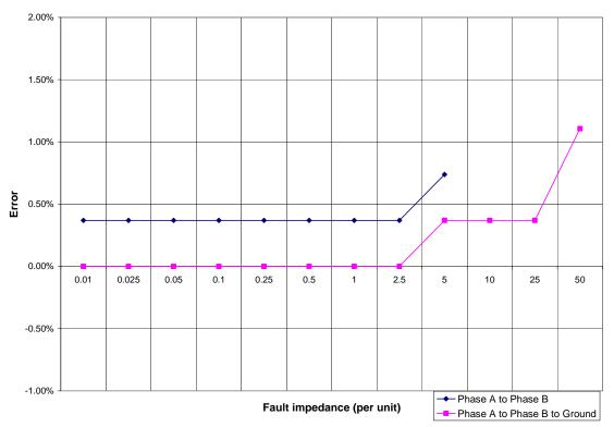
Figure 5-4 - Fault location error as a function of fault impedance for line to line faults
