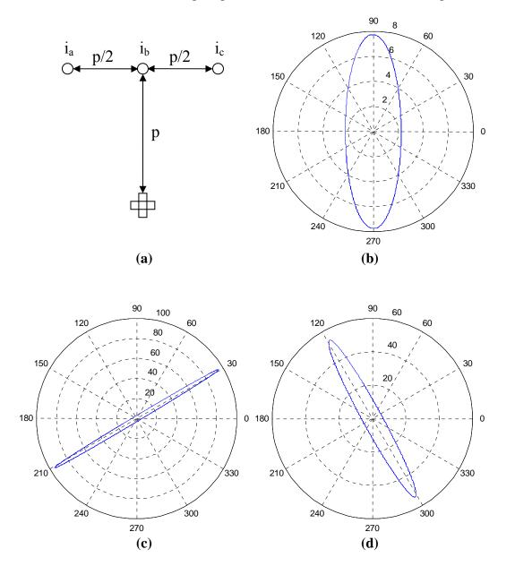
Figure 3-4 – Horizontal conductor configuration and plots of its magnetic field
