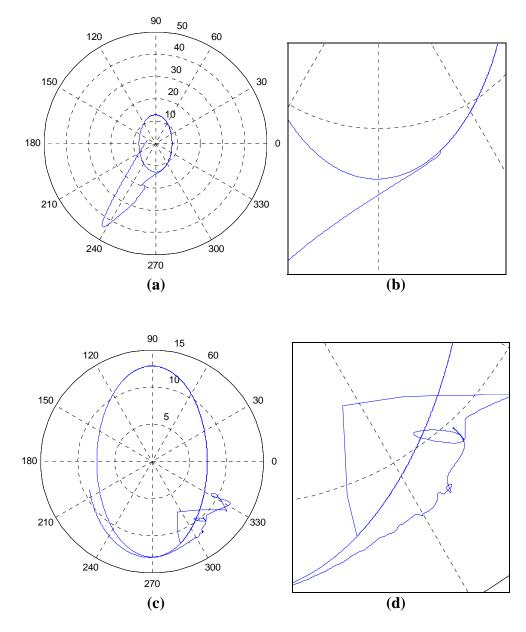
Figure B-2 – Line-to-Ground Fault: Phase a, fault connected at phase a current peak
