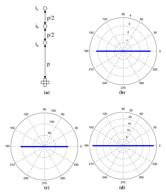
Figure 3-8 – Vertical conductor configuration and plots of its magnetic field (a) – Conductor geometry; (b) – Magnetic field for balanced currents, p=2m; (c) – Magnetic field for a line to ground fault on phase a, p=2m; (d) – Magnetic field for line to line fault on phases a and b, p=2m
