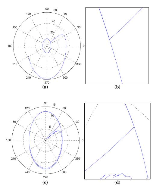
Figure B-6 – Three Phase Fault (a) – Generator end magnetic field; (b) – Generator end magnetic field fault detail; (c) – Load end magnetic field; (d) – Load end magnetic field fault detail
