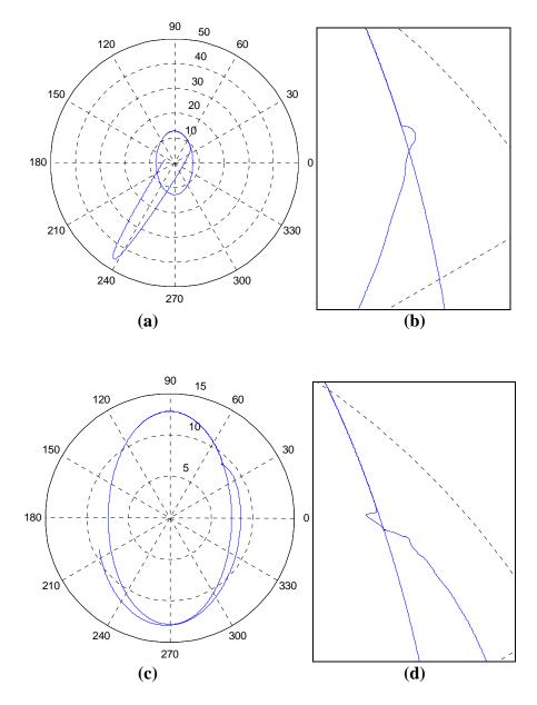
Figure B-3 – Line-to-Ground Fault: Phase a, fault connected at phase a current zero-crossing (a) – Generator end magnetic field; (b) – Generator end magnetic field fault detail; (c) – Load end magnetic field; (d) – Load end magnetic field fault detail
