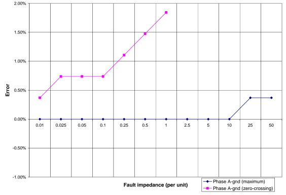
Figure 5-3 – Fault location error as a function of fault impedance for single line to ground faults
