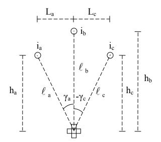
Figure 3-3 – Variables for magnetic field analysis of a three-phase system
