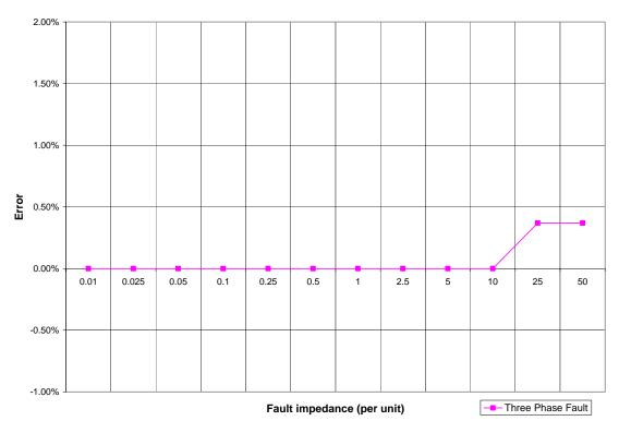
Figure 5-5 – Fault location error as a function of fault impedance for three phase faults
