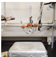
Figure 3.1 The initial set up of the MXene surface silanization, with inlet of Argon on the right arm, Argon outlet on the left arm, and the silane syringe in the center. The stir bar is present in the three-neck flask, and from this distance the stir bar would mix the solution.
