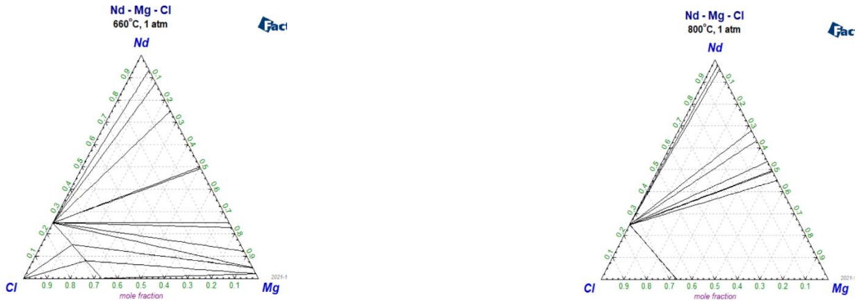
Figure 12: Nd-Mg-Cl phase diagrams at 660°C (left) and 800°C (right) showing Mg-Nd alloy with low Nd concentration in equilibrium with MgCl 2 -NdCl 3 salt having high Nd concentration.
