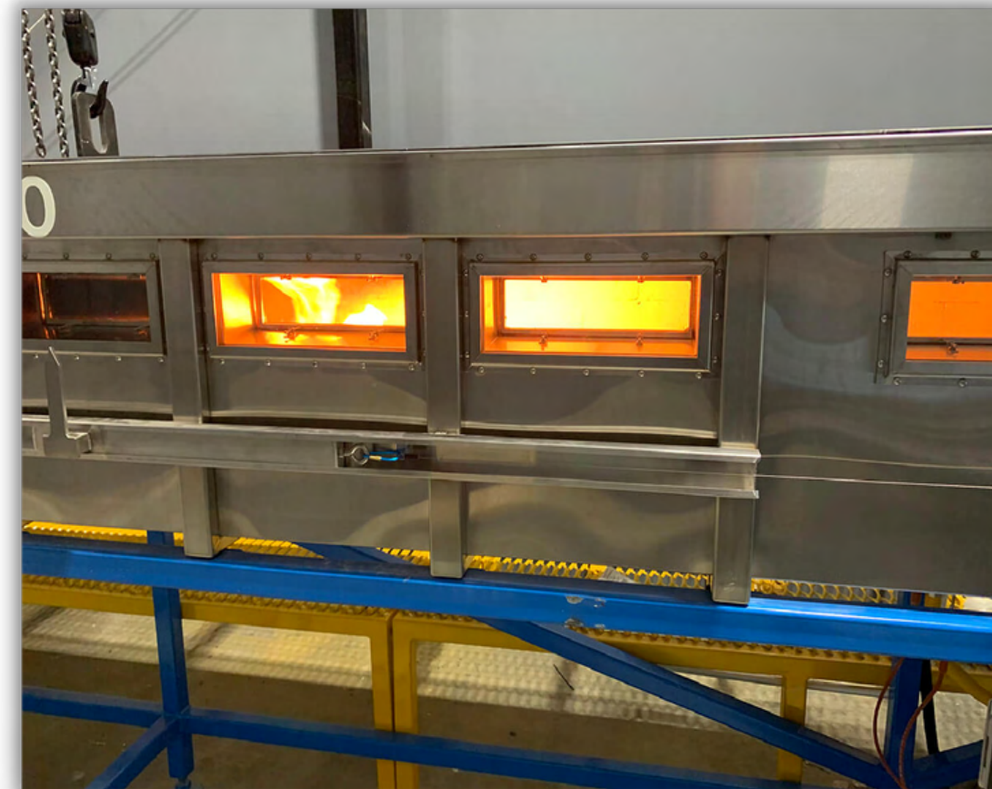
Figure 14: Photograph of ASTM E84 tunnel test for flame spread index value. (ICC NTA, 2022)
