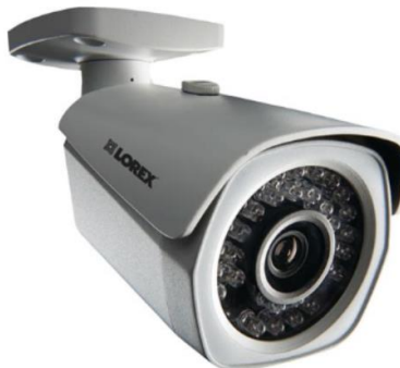
Figure 4.7. A common internet protocol camera (Amazon Lorex 1080P IP Camera, n.d.)
