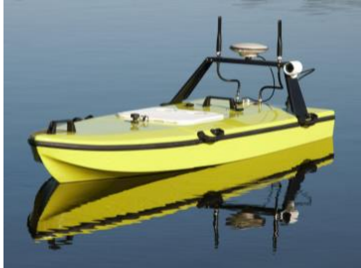
Figure 2.9. CEE-USV Autonomous Boat (CEE-USV / CEE Hydrosystems, n.d.)
