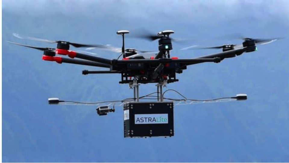
Figure 2.10. ASTRALite UAV (“ASTRALiTe Edge, First Small-Scale LiDAR for Underwater Exploration,” 2019)
