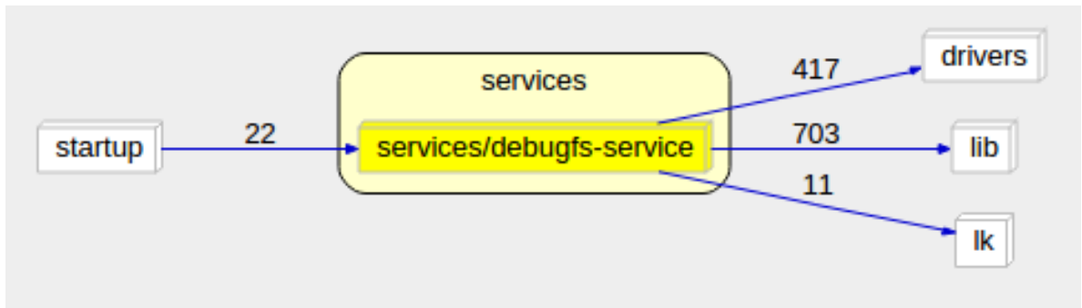
Figure 3.2: A butterfly dependency graph generated by SciTools Understand after the debugfs interface code was fully segregated.
