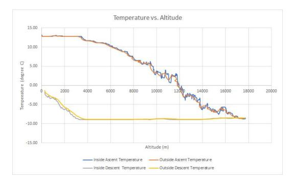
Figure 17: Temperature vs. Altitude
