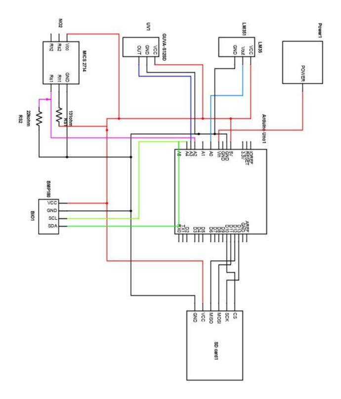
Figure 4: Arduino Uno 2 Schematic
