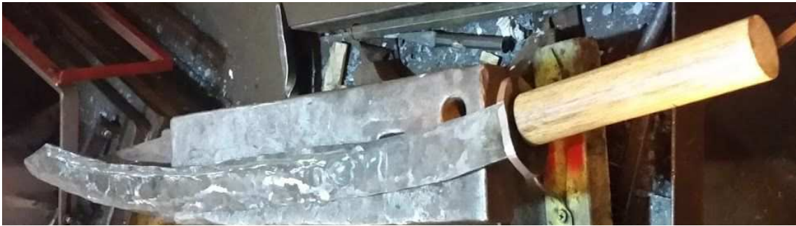
Figure 37. The assembled dao at of the eleventh day of forging.
