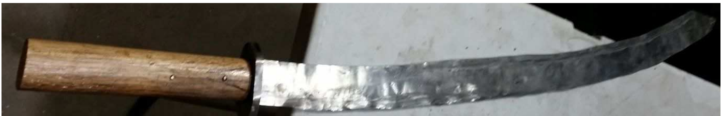
Figure 39. The assembled dao before quenching and tempering.
