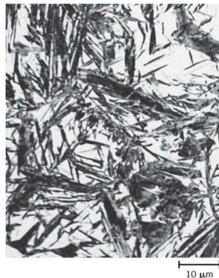
Figure 55. Image of martensite microstructure [3].
