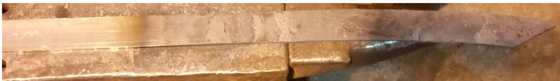
Figure 25. Full-sized actual dao at the end of Day 3 of forging.
