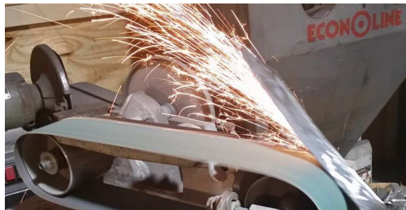
Figure 31. Grinding the larger dao.
