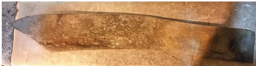
Figure 24. The practice dao after quenching.
