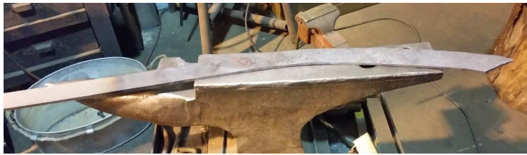
Figure 26. Full-sized actual dao at the end of Day 4 of forging.
