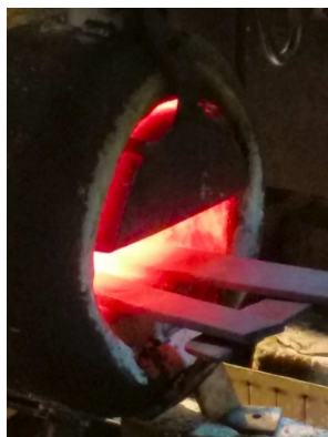
Figure 17. The scrap metal being heated in one of the forges.
