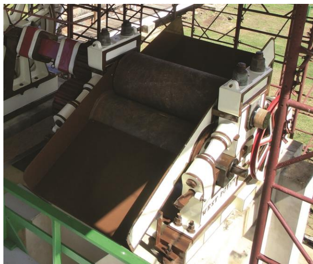
Figure 1. The large rollers that crushed the cane
