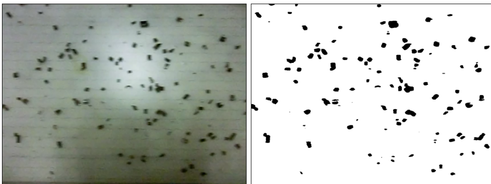
Figure 4: Comparison of image extracted from feeding video (left) and converted into a binary image (right).
