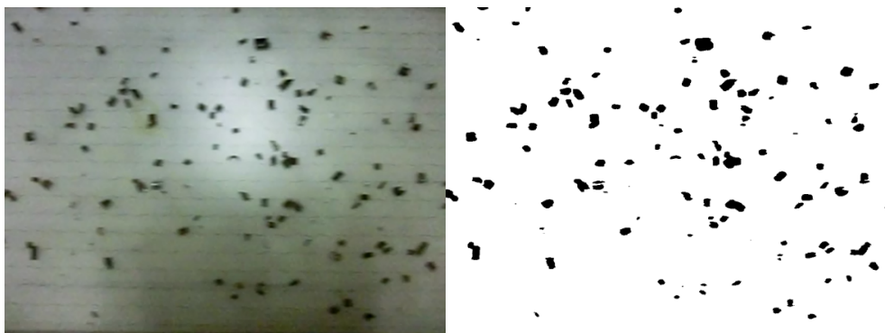
Figure 7: Comparison of image extracted from feeding video (left) and the converted binary image (right).
