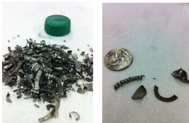
Figure 11: Morphology of Ti-64 chips.
