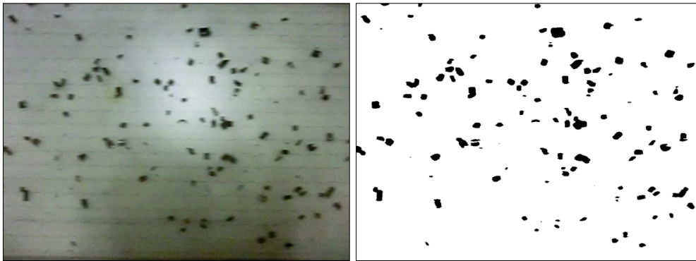
Figure 14: Comparison of image extracted from feeding video (left) and the converted binary image (right).
