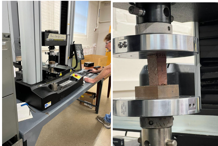
Figure 8. Universal Testing Machine Compression Testing Set-Up
