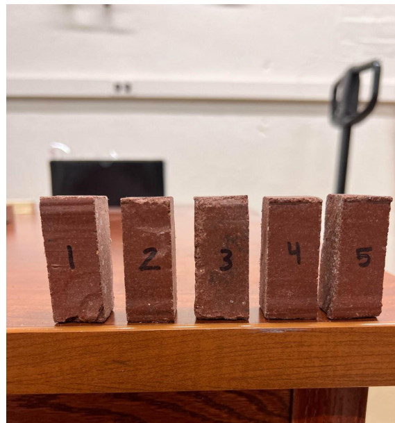
Figure 7. EcoBlock Samples #1-5 Before Compression Testing
