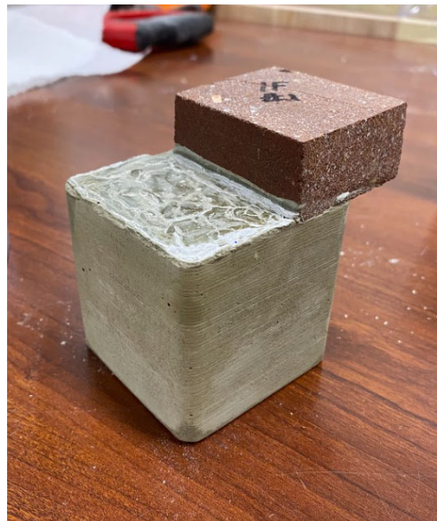
Figure 11. EcoBlock Sample Bonded to Concrete Before Testing.
