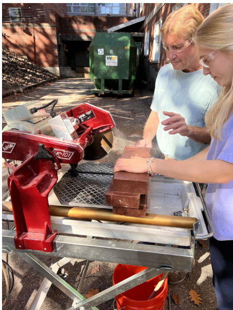
Figure 6. EcoBlock Sample Preparation for Testing
