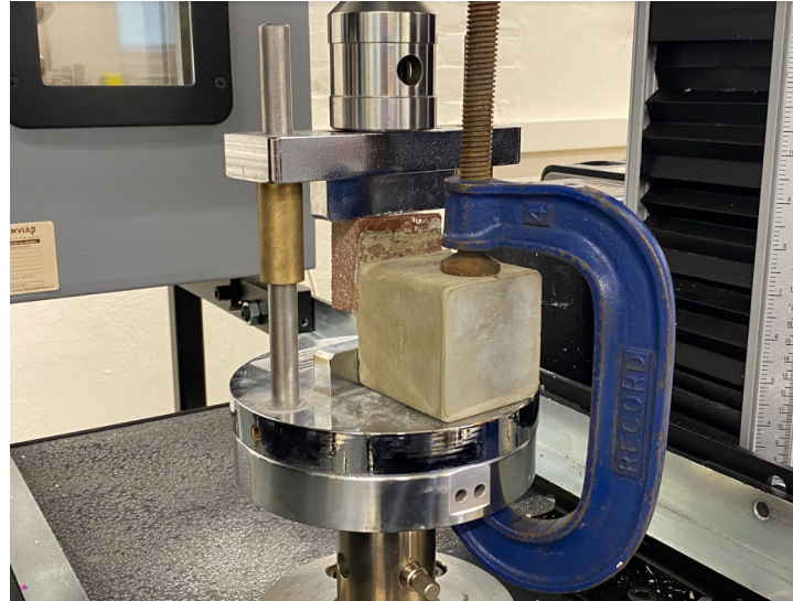
Figure 12. Universal Testing Machine Shear Strength Test Set-Up.
