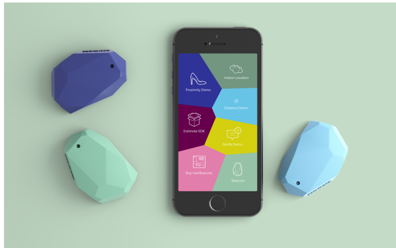
Figure 2: Three Estimote Proximity Beacons and the main user interface of the Estimote mobile application. [Estimote]
