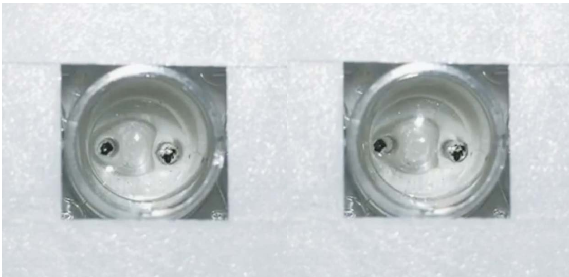
Figure 18. Relaxed state of PDMS posts.
