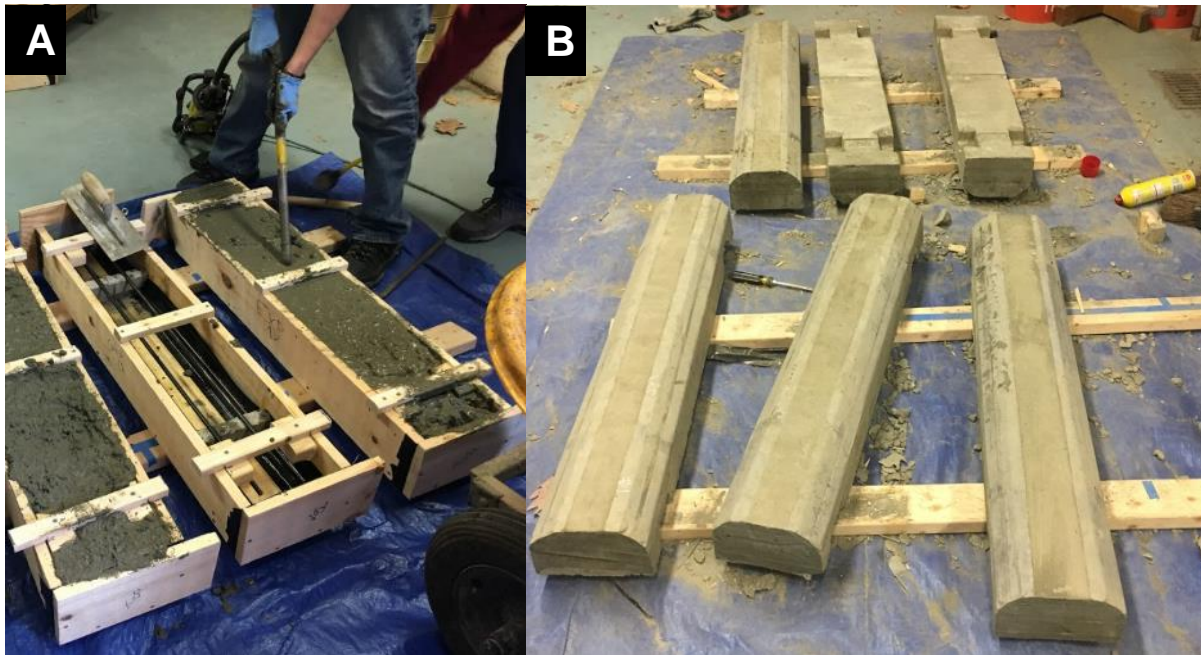
Figure 12. (a) Concrete vibration tool operated on filled mold. (b) Concrete stops after 24 hours.
