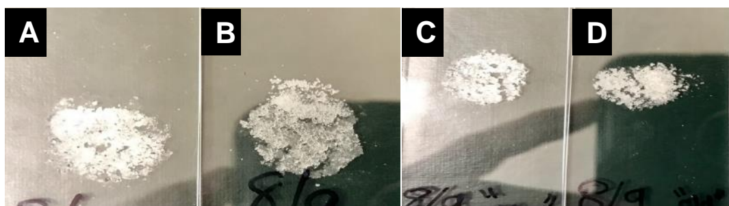
Figure 24. Liquid tung oil present in S1. (a) Fresh capsules. (b) Capsules allowed to oxidize one week. S1 was replicated because the amount of liquid tung oil was equal in both cases. (c) Retest of fresh capsules. (d) Retest of capsules allowed to oxidize one week.
