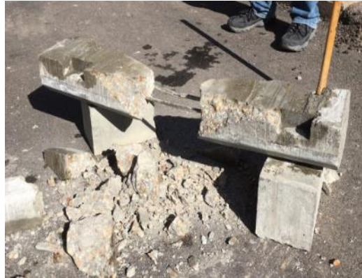
Figure 14. Three-point bending system for concrete stop damage.
