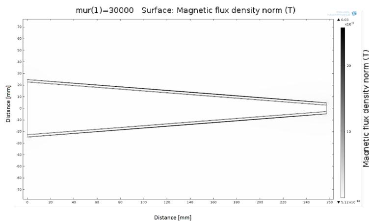
Figure 2: COMSOL computation for 2 layers: Top: Close look at the exit Bottom:Plot showing magnetic field strength density, ranging from 0.5G, the background magnetic field to about 300G.
