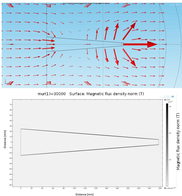
Figure 1: COMSOL computation: Top: An Arrow Plot of the magnetic field lines Bottom:Plot showing magnetic field strength density, ranging from 0.5G, the background magnetic field to about 300G.
