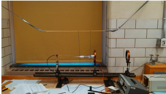
Figure 4: Photo of the cone being suspended from a dowel.
