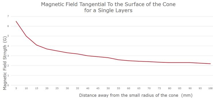
Figure 6: Plot of the data points taken for a single layer of the material
