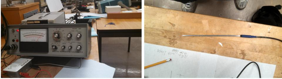
Figure 3: Tools used for measurements Left: Bell Model 640 analog Gaussmeter. Right: Transverse Hall Effect Probe.
