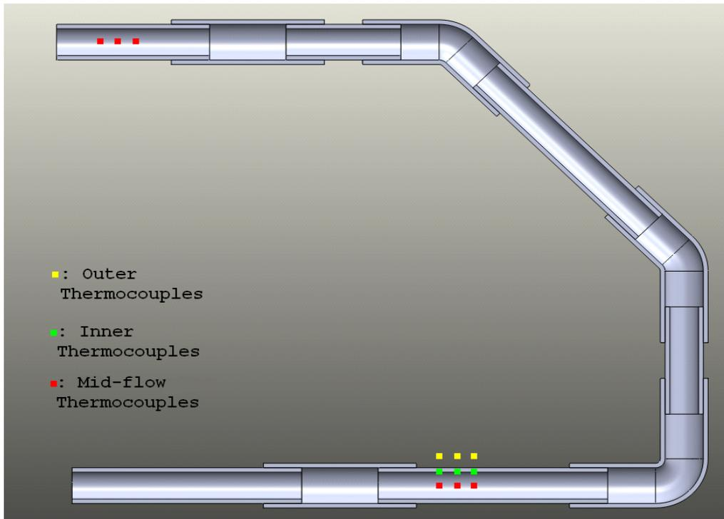
Figure 7 : Cross Section View of Test Rig with Thermocouple Placement
