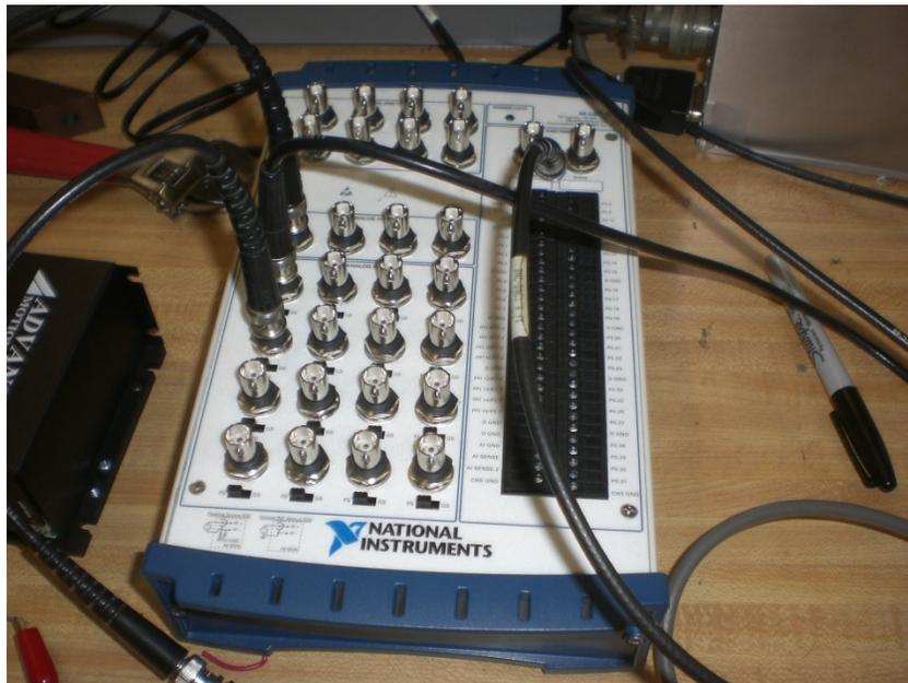
Figure 15 : Data Acquisition Board Used During Testing
