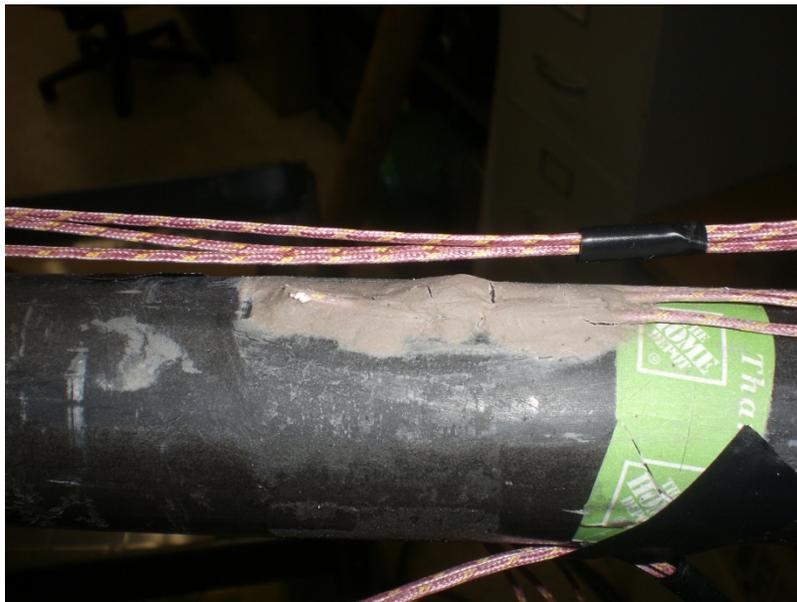
Figure 12 : Upper Midflow Thermocouples Secured via Furnace Paste
