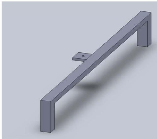
Figure 5 : SolidWorks Rendering of Fire Grate Support Legs Concept
