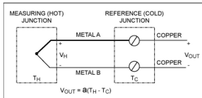
Figure 6 : Thermocouple Schematic
