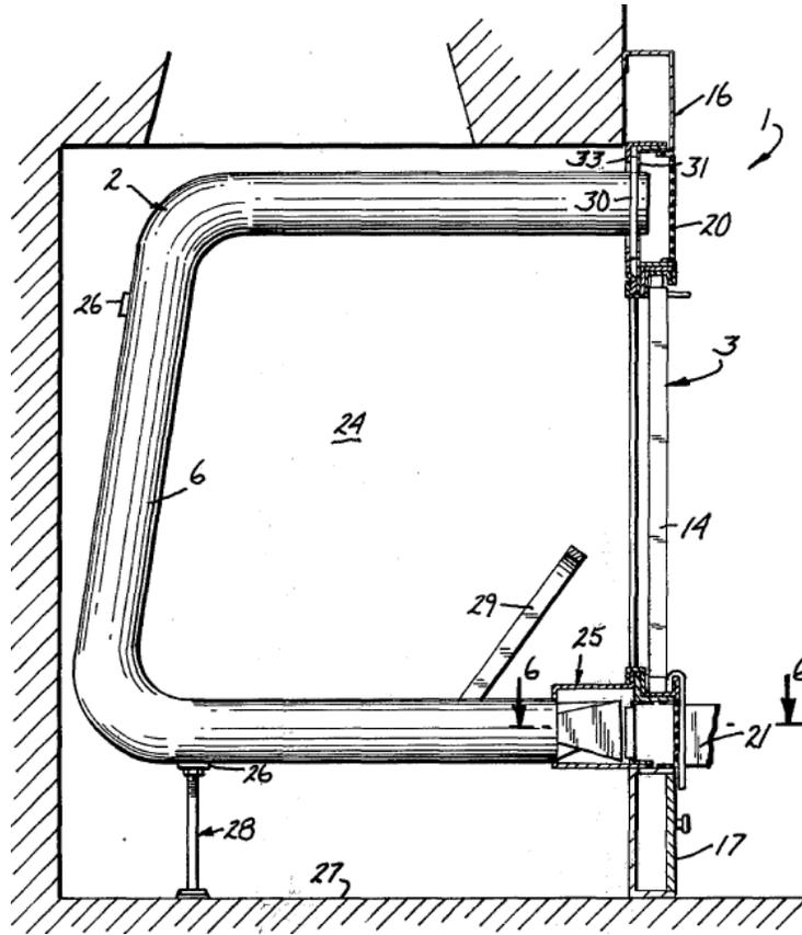
Figure 2: Side View Schematic of U.S. Patent 4,129,113 - Example of a Vertical Fireplace Grate with Glass Door Faceplate (Bergstrom, 1977)
