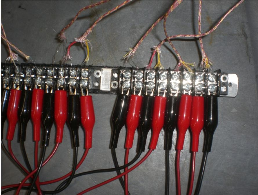
Figure 17 : Screw Terminal Thermocouple Wiring
