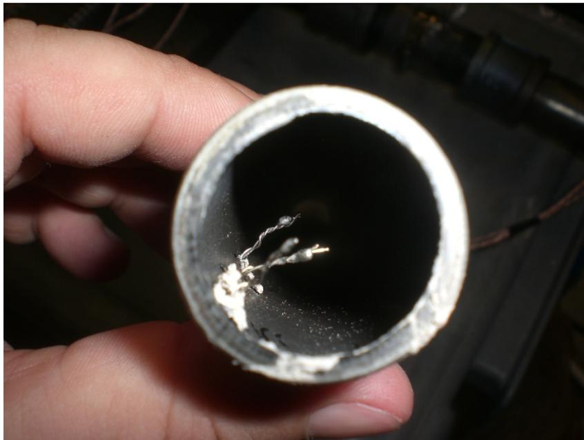
Figure 10 : Inner Pipe Midflow Thermocouples Located Near Pipe Entrance
