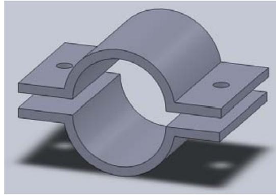
Figure 4 : SolidWorks Rendering of Pipe Securing Clamp
