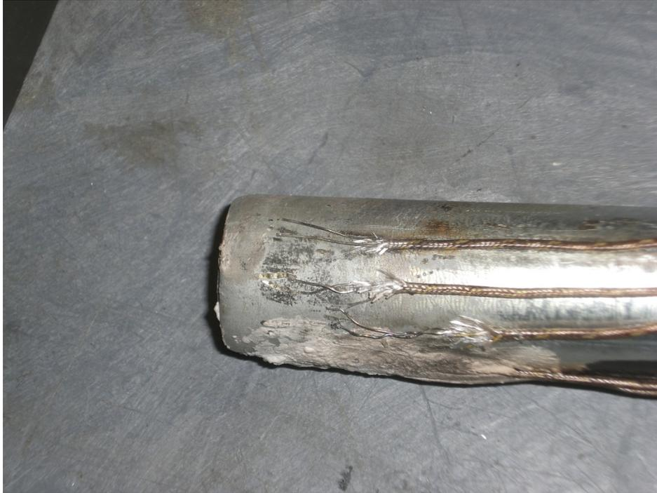
Figure 9 : Inner Pipe Thermocouple Layout
