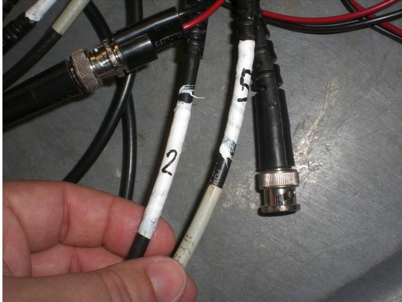
**Figure 16 : Labeled BNC Cables Attached to DAQ Board**
