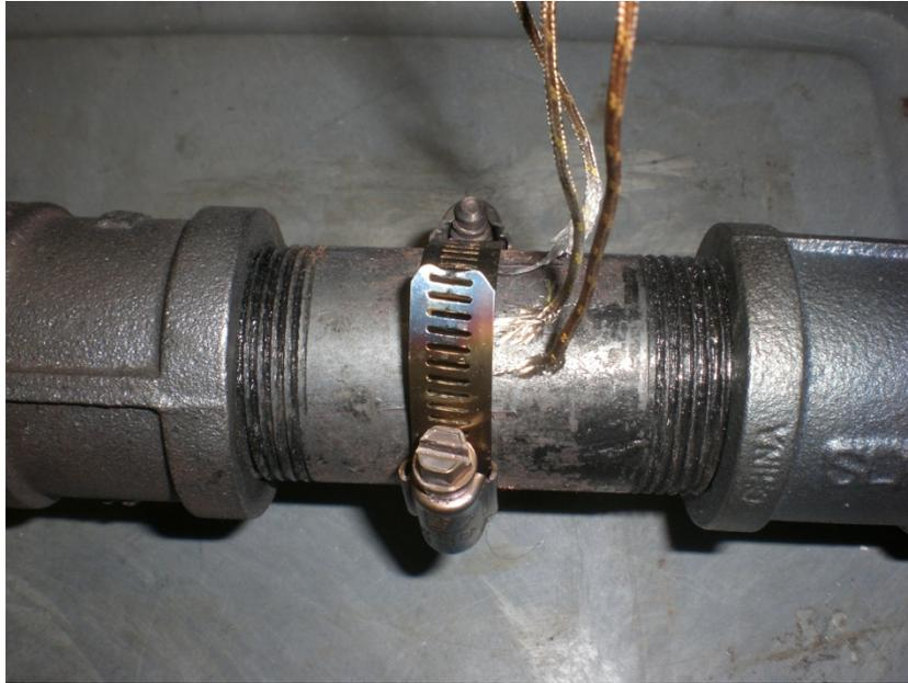
**Figure 8 : Outer Thermocouple Configuration Close Up**
