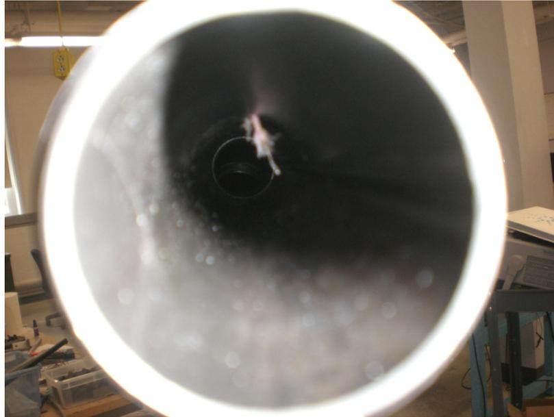
Figure 11 : Midflow Thermocouples Located Near Pipe Exit
