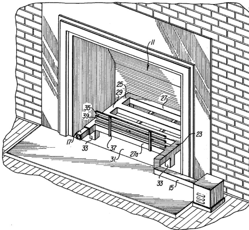
Figure 1: Schematic of U.S. Patent 4,010,729 - Example of a Horizontal Fireplace Grate with Blower (Egli, 1975)
