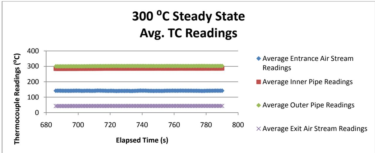
Figure 21 : 300C Test Temperature vs. Time
