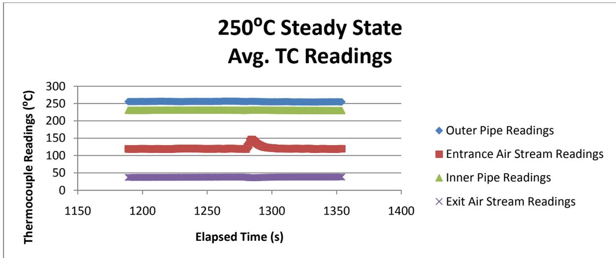
Figure 20 : 250C Test Temperature vs. Time
