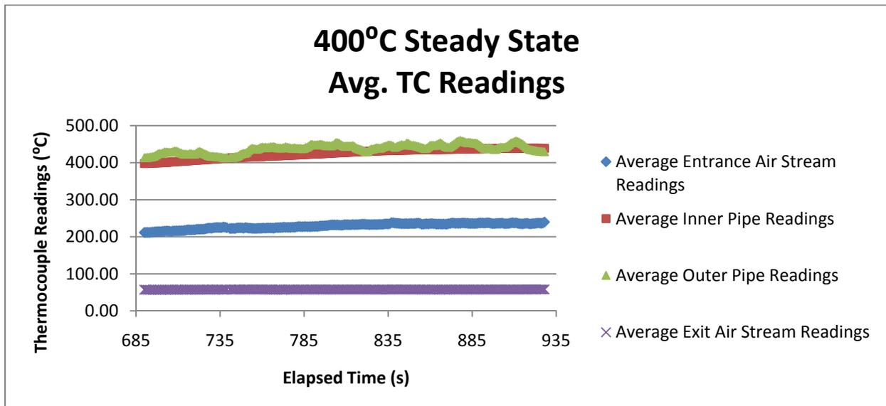
Figure 22 : 400C Test Temperature vs. Time
