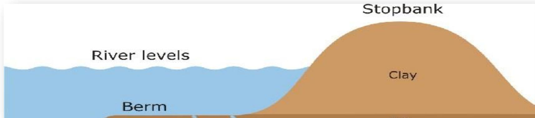
*Figure 2: Cross section of a river with a stopbank. Adapted from Waikato Regional Council.*
