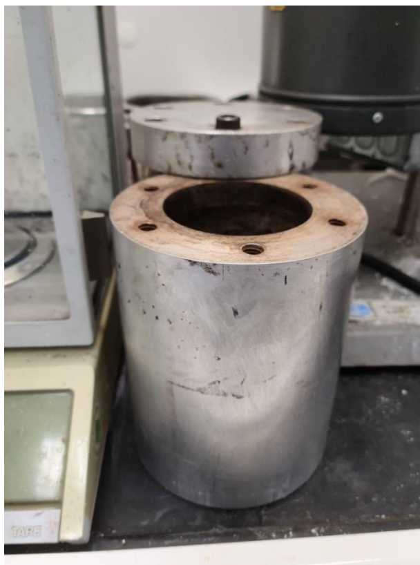
Figure 6: Steel autoclave where Teflon inlet was placed for heating in oven
