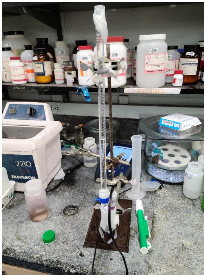
Figure 13: Boehm titration experimental setup
