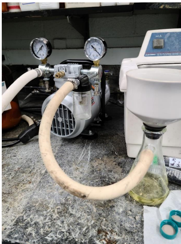
Figure 7: Vacuum filtration setup for separating solid from aqueous phase
