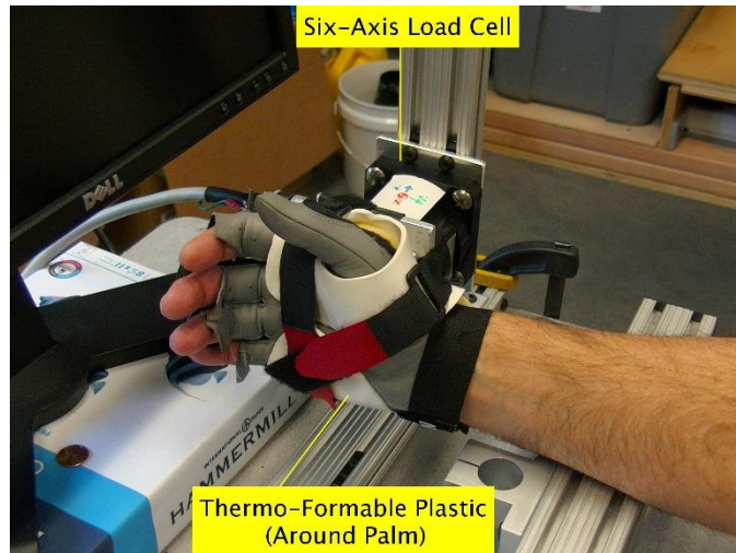
Fig. 6.1. Experimental apparatus. Dominant hand was tightly secured via thermo-formable plastic and Velcro to six-axis load cell. Sixteen electrodes (not visible) were secured about the distal aspect of the dominant forearm.
