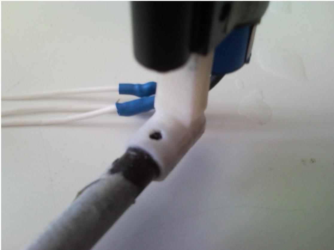
**Figure 18.a-Gaps in FDM Modeled Motor Mount**
