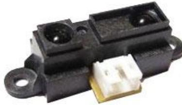
**Figure 5-Sharp GP2D12 Infrared Rangefinder**
