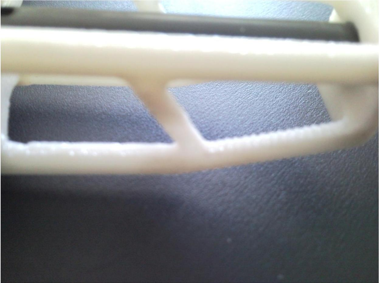
**Figure 23.b Gaps and "Stepped Edges" on FDM Central Hub**
