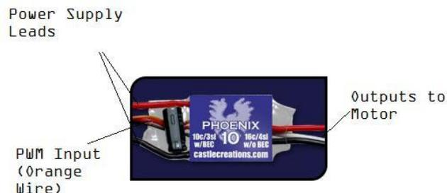
Figure 20-Speed Controller Hookup Diagram
