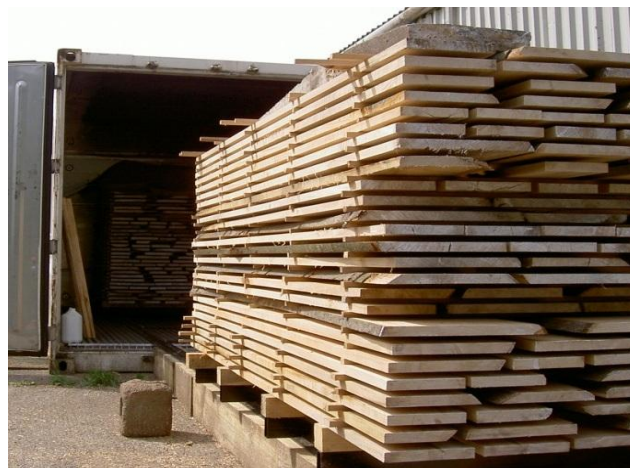
Figure 2.4- 1: Wood Stacking and Drying ( http://www.lumberbylance.com/kiln.php )
