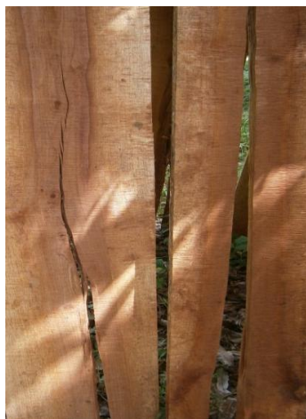
Figure 4.2- 10: Cracks in Plantation Pochote Timber
