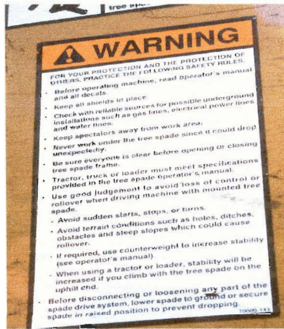
Figure 4: Warning sign for proper procedure while using tree spade.
