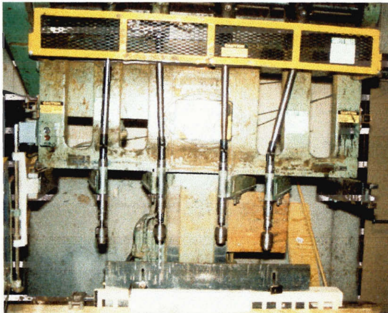
Figure 1: Unguarded boring machine showing highly exposed spindles.
