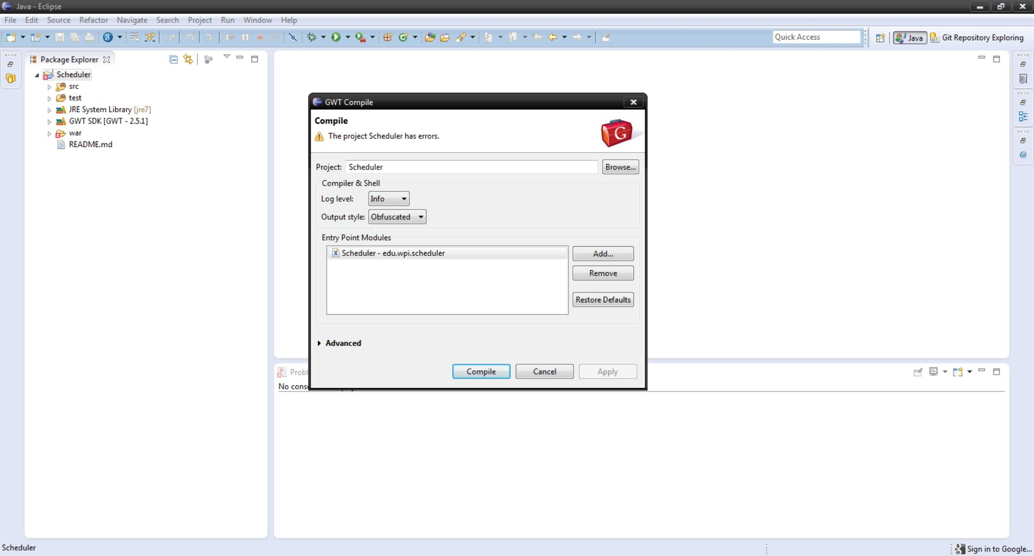
There are some files that are not automatically generated unless you edit and run the project; however, these missing files do not affect the project from being compiled properly, so the warning is safe to ignore. The default compilation settings are fine for hosting purposes. There is no need to edit them unless you have a particular reason to.
