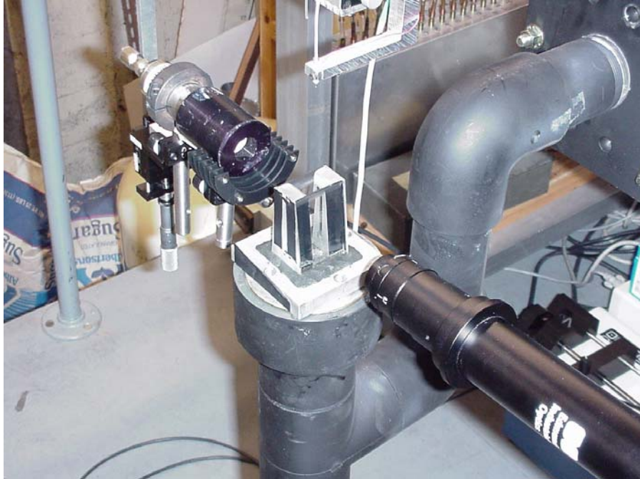
Figure 2.1 Photograph of high-magnification imaging configuration. Top left corner: Nanopulser. Bottom right corner: VZM lens and Panasonic CCD camera.
