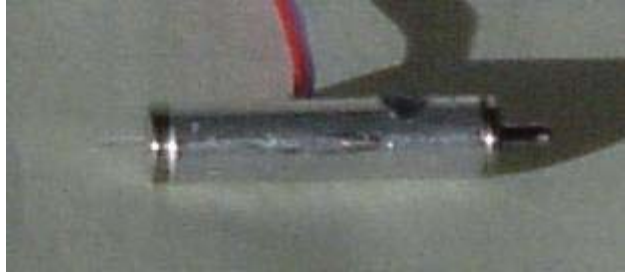
Figure 2.5 Photograph of DoD Dispensing Device. The fluid supply is attached to the metal nib on the right hand side of the image and droplets are ejected from the glass tip on the left hand side of the image. The dispensing device is 0.5 inch (12.7 mm) long.
