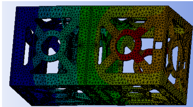
Figure 20. Total Deformation Occurring at Mode 3
