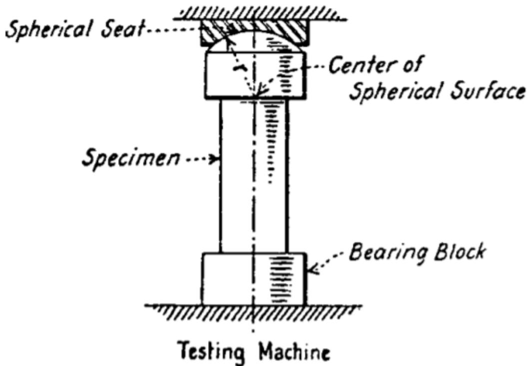
**Figure 4: Compressive Bearing Block Illustration I**
