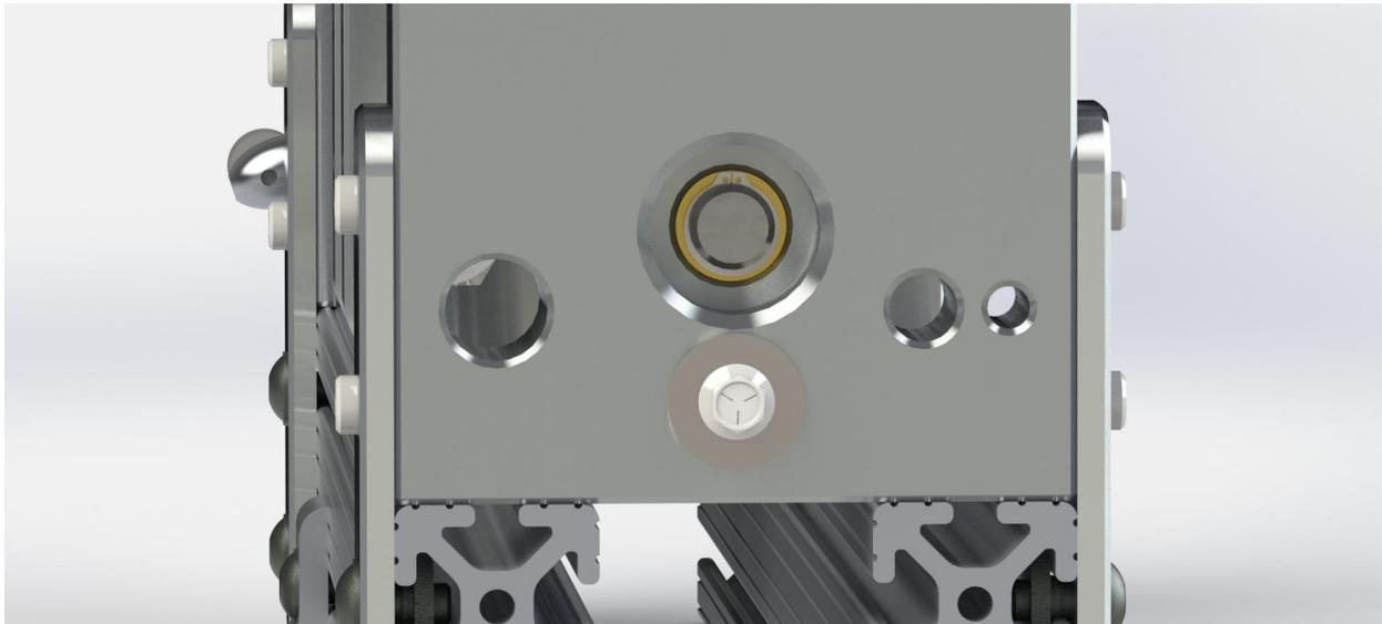
**Figure 15: Outside Fixturing of Round Samples to Crossheads CAD**
