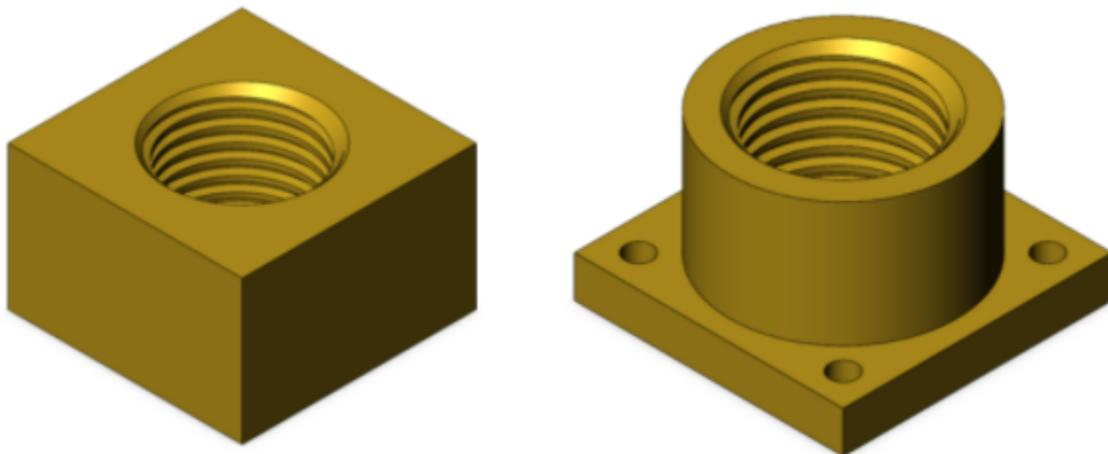
**Figure 13: Brass Nut as Purchased (Left) and After Machining (Right) CAD**
