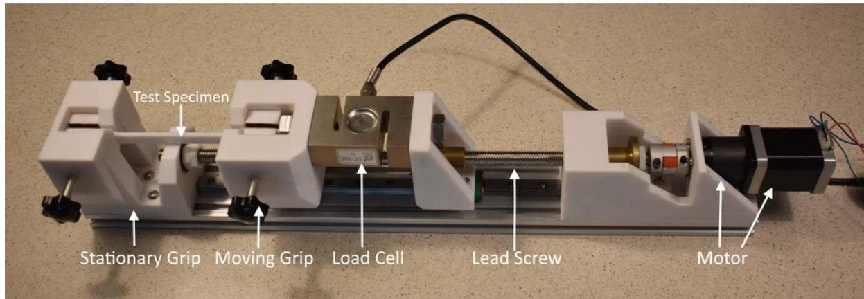
**Figure 1: Example of a Horizontally Oriented Materials Tester**
