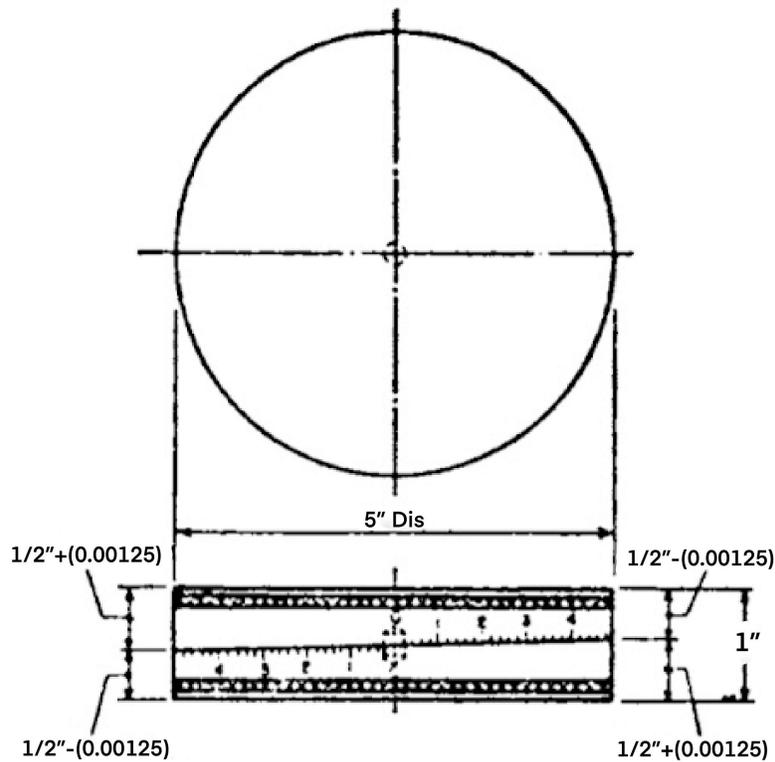
**Figure 5: Compressive Bearing Block Illustration II**
