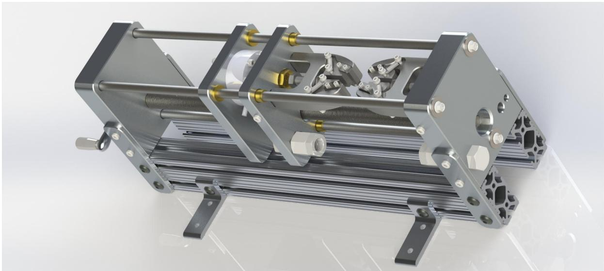
**Figure 11: CAD Model of Universal Materials Tester Prototype Design**
