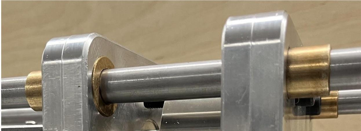
**Figure 31: Bronze Oilite Bearings on Linear Motion Rods & Crossheads**
