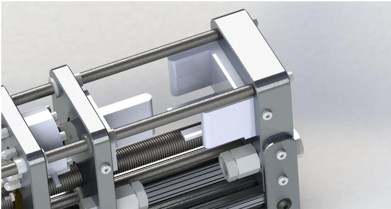
**Figure 20: Preliminary CAD Design of Three-Point Bending Grips**
