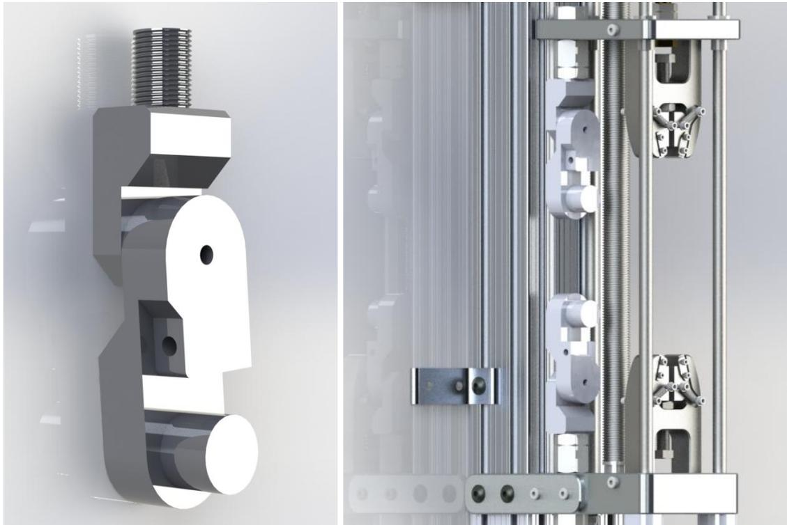
**Figure 19: Preliminary CAD Design of Wire Sample Grips**
