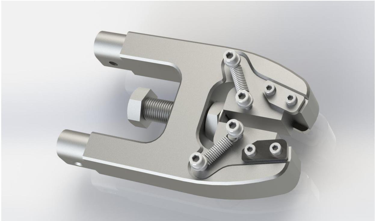
**Figure 17: Flat Sample Grips CAD**
