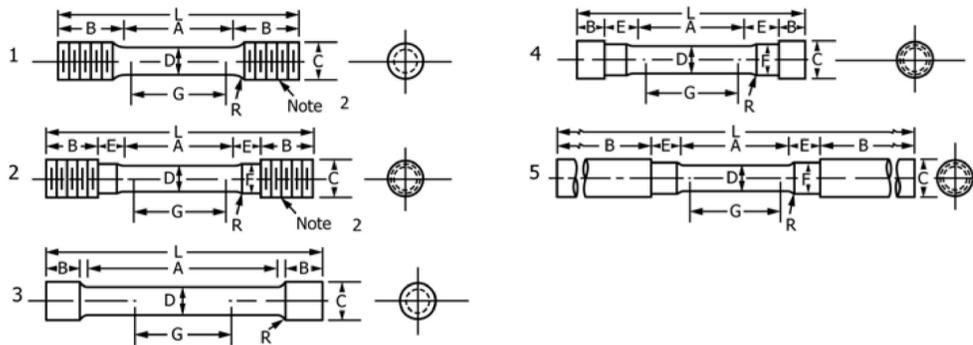
**Figure 14: Free-Form Round Sample Processing**
