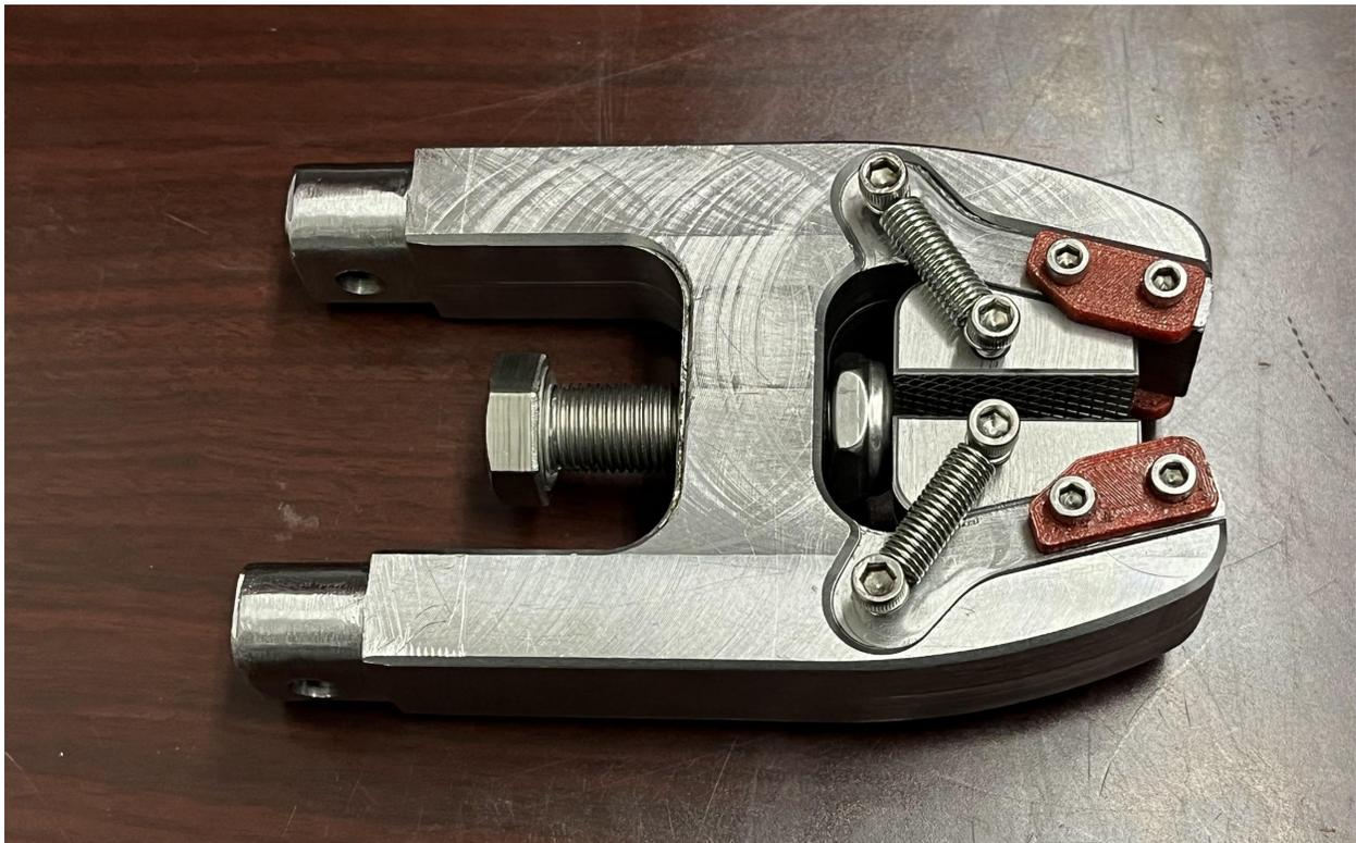
**Figure 33: Completed Flat Sample Grips**
