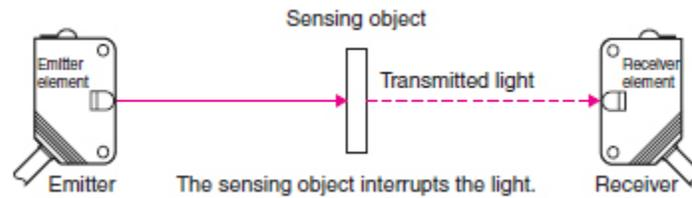
*Figure 4 Through-beam Sensors*
