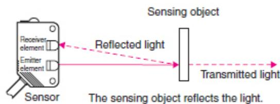
*Figure 6 Diffuse-reflective Sensors*
