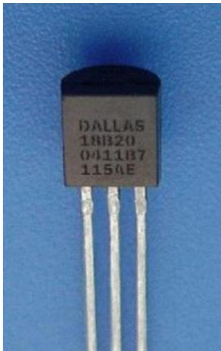
*Figure 9 The Temperature sensor used in the device*
