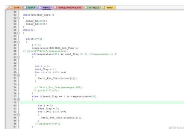
Figure 12 Code for STM circuit board, which reads the temperature sensor and sends the respective data to the OpenMV
