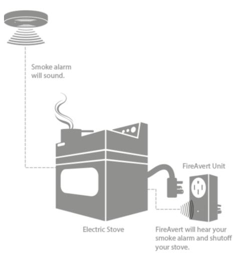
Figure 8 Automatic stove shut-off device.
