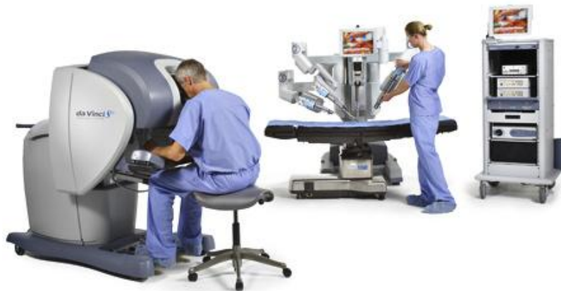
Figure 2.1: Da Vinci Teleoperated Surgical System. Pictured at the left is the master controller manipulated by the operator, to the right is the slave robotic manipulator ( Intuitive Surgical ).
