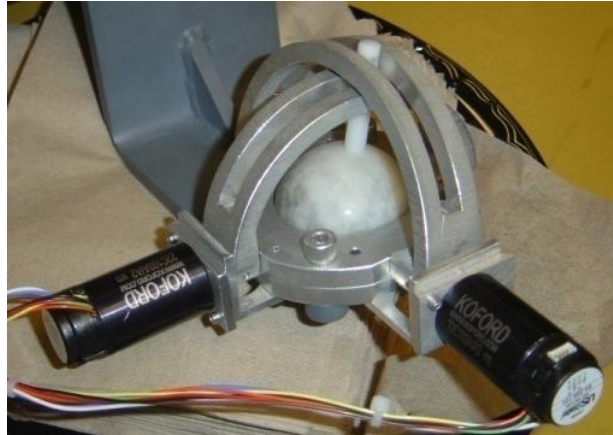
Figure 5.13: Inspiration for the design of the spherical wrist came from a device to emulate eye movement.
