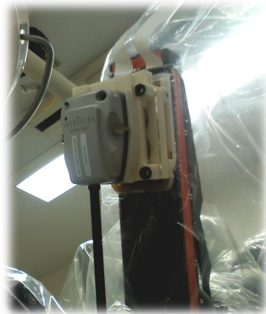
Figure 2.1: Sensor module on da Vinci Surgical robot at Children’s Hospital Boston, confirming design objective
