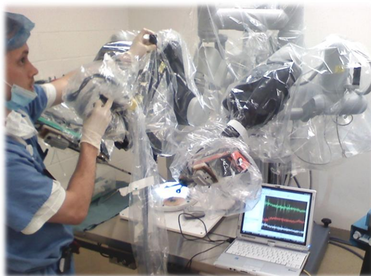
Figure 6.2: Further confirmation of device functionality, the arm was moved while the sensor module was attached.
