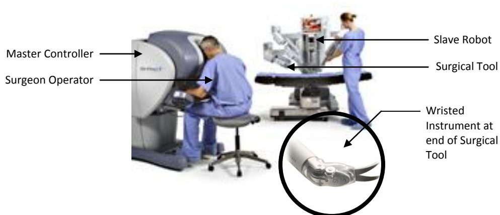
Figure 1.1: Components and layout of master-slave robot-assisted surgery. Specifically, the da Vinci Surgical System is pictured ( Intuitive Surgical ).
