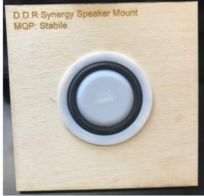
FIGURE 89: SPEAKER VIBROMETER MOUNT, FRONT VIEW
