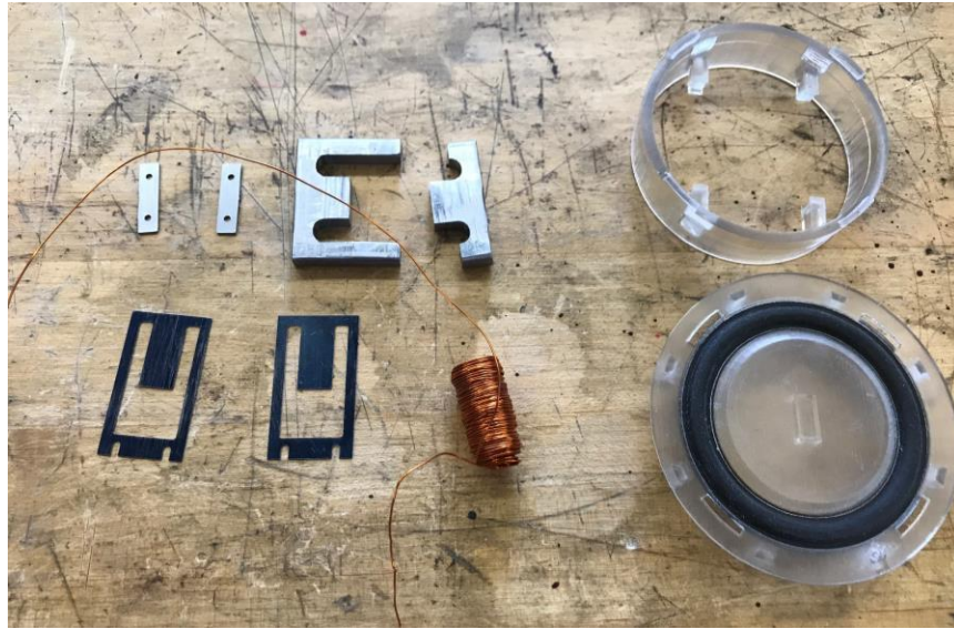
FIGURE 24: COMPONENTS OF MOVING MAGNET TRANSDUCER
