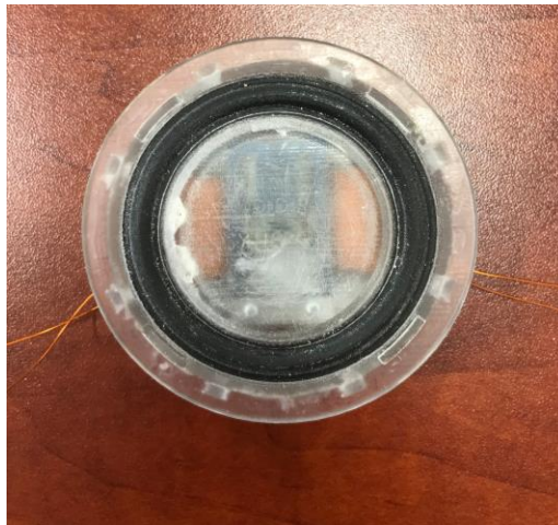
FIGURE 68: CONNECT TOP HOUSING AND CONE WITH GLUE
