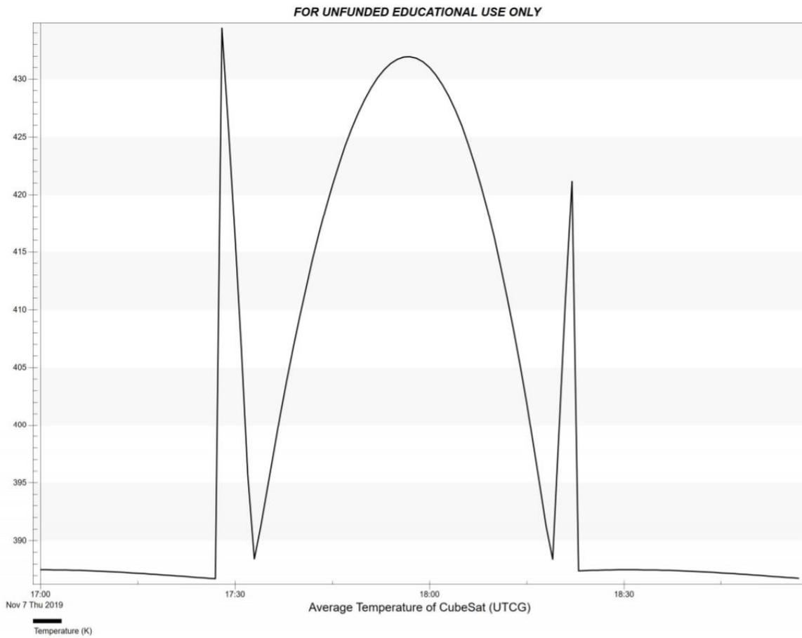
**Figure 52b: Average Temperature over One Orbit**
