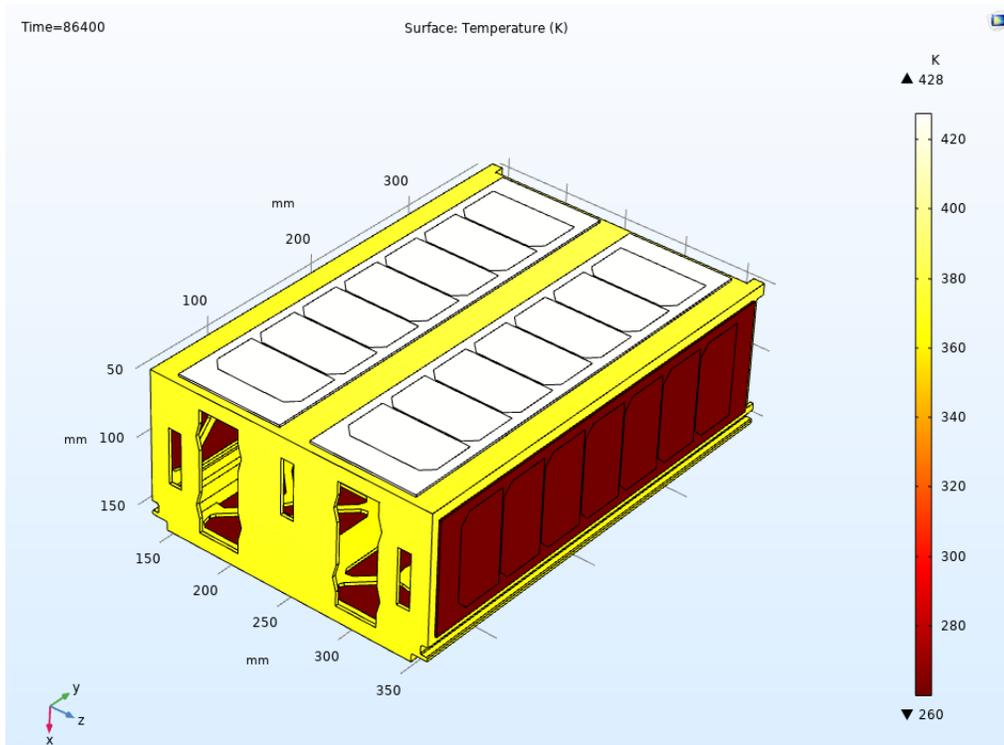
**Figure 50a: NeAtO Temperature Profile after 24 Hours in Orbit (View 1)**
