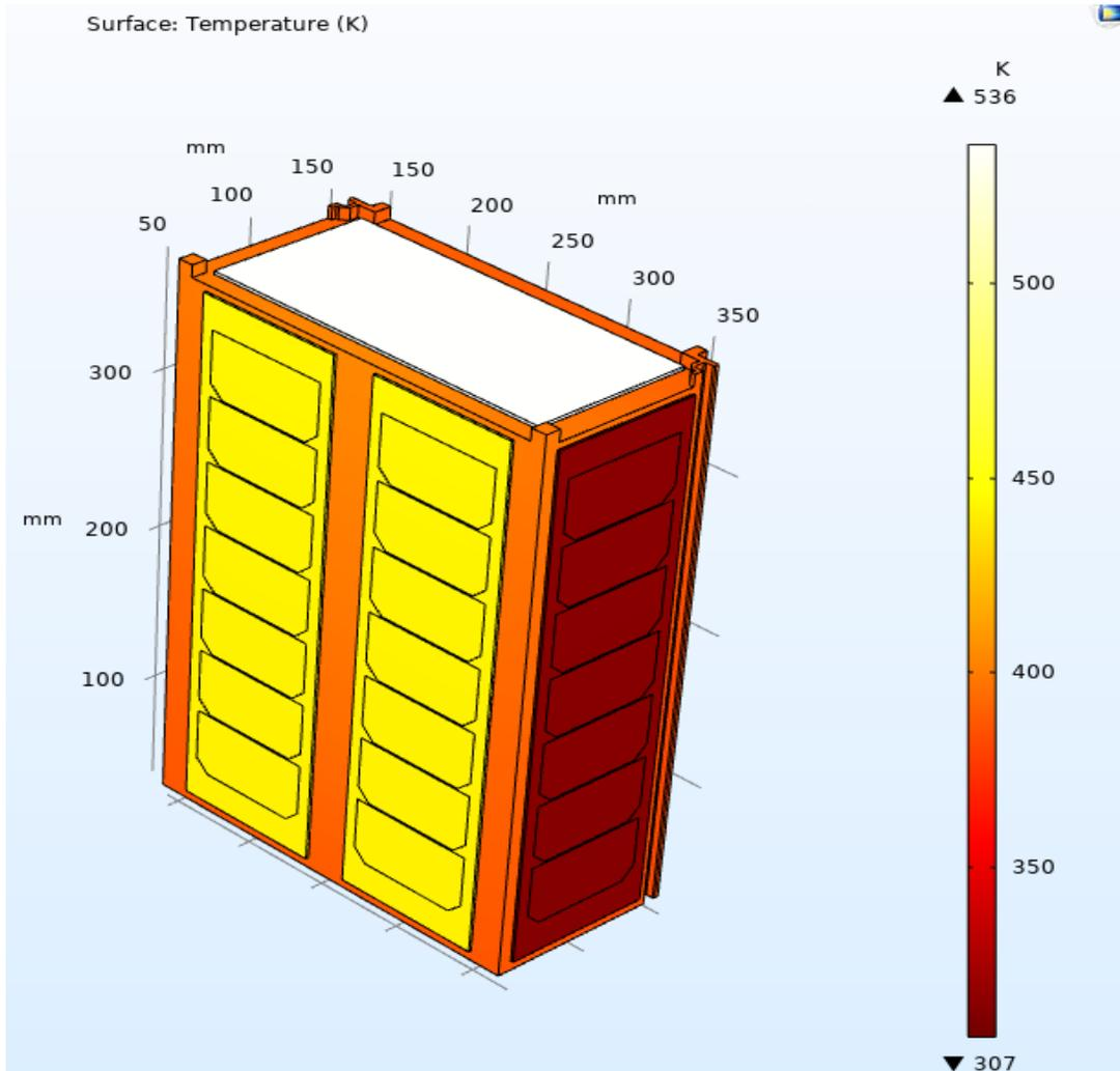
**Figure 49b: NeAtO Temperature Profile Modelled with a Front Plate (View 2)**
