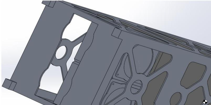
**Figure 22: Thruster Mount - only exists -Z Face**
