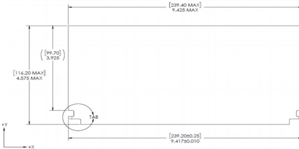
**Figure 16: Tab Dimensions with Respect to X and Y axis' [23]**
