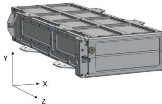
Figure 14: NanoRacks Deployer Coordinate System [23]
