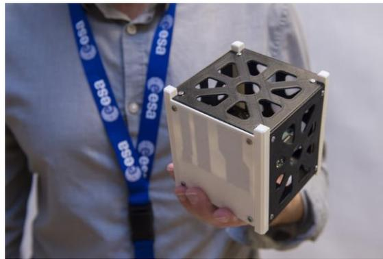
**Figure 1: 1U CubeSat Frame [5]**
