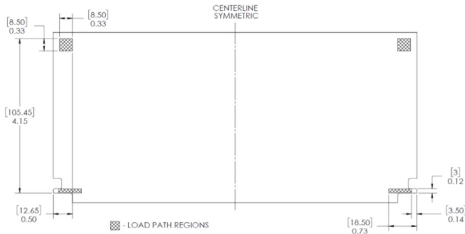
Figure 18: Load Points for Tab Configuration [23]
