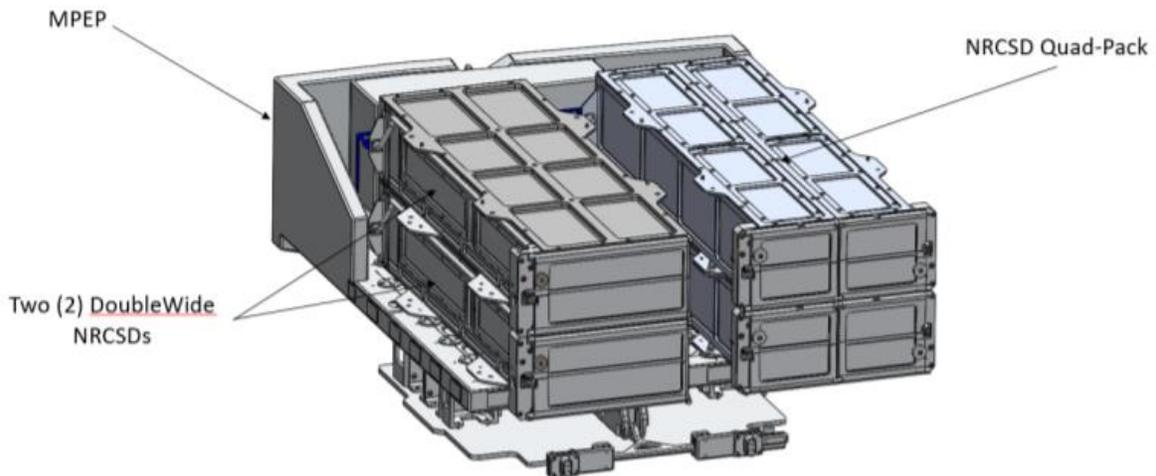
Figure 10: NRCSD Standard and DoubleWide Deployers [23]
