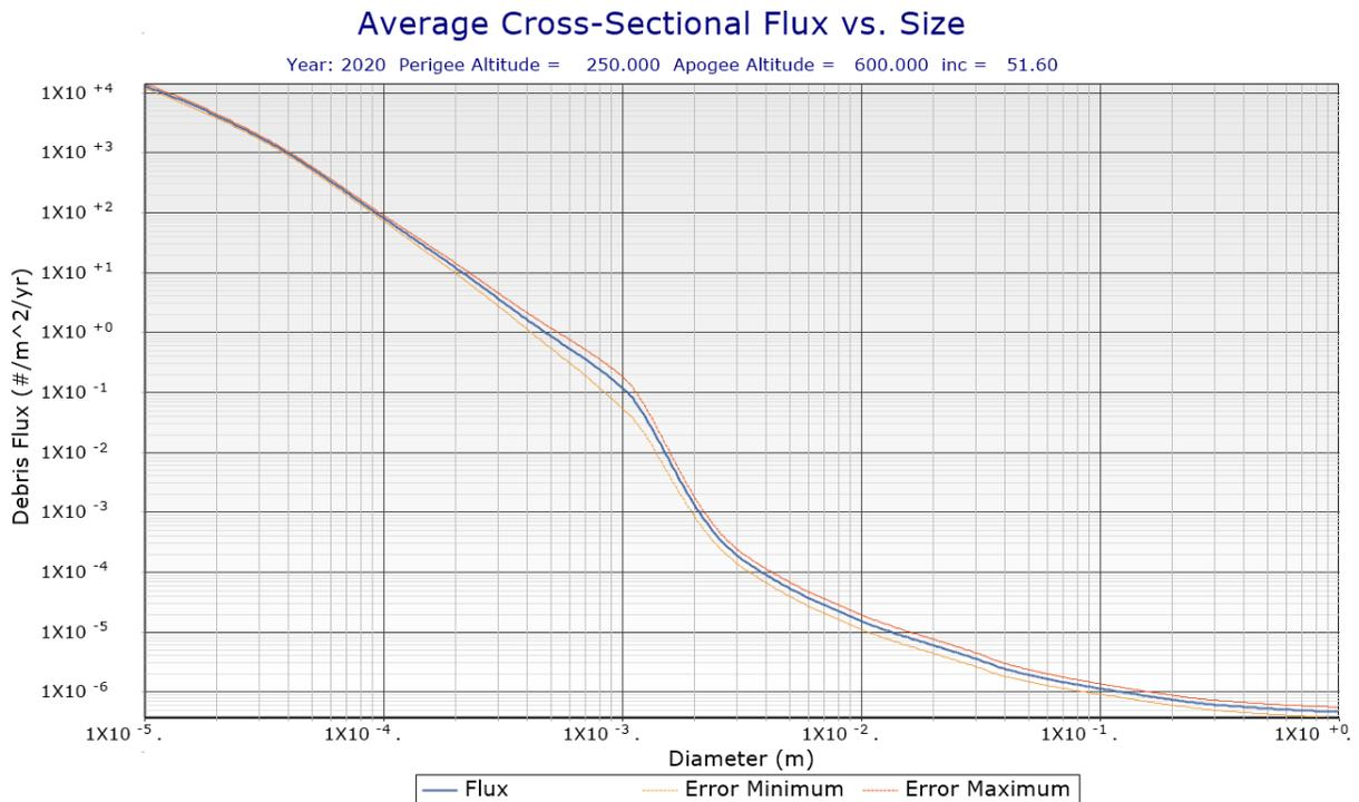
**Figure 40: Debris flux vs Diameter**
