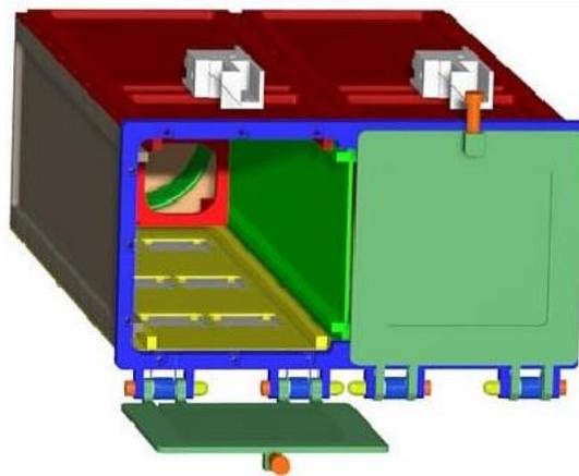
**Figure 7: Illustration of P-POD Double Deployer (2x3U), [18]**
