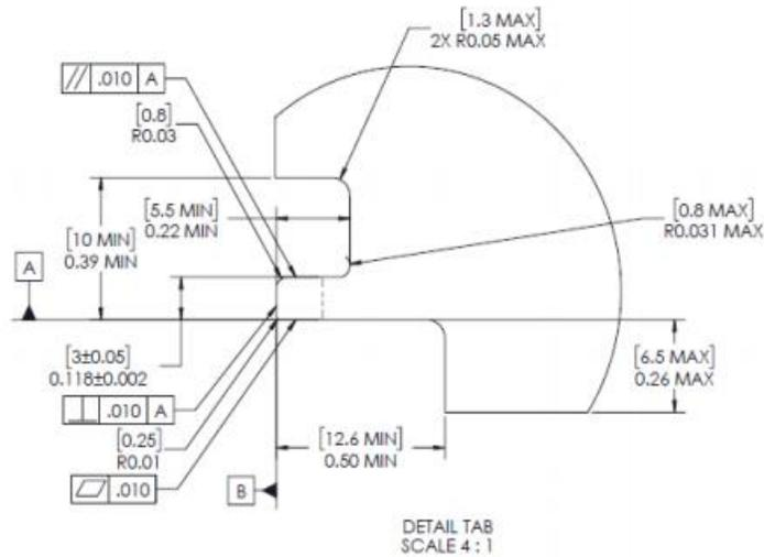
Figure 17: Tab Dimensions: Close-Up [23]
