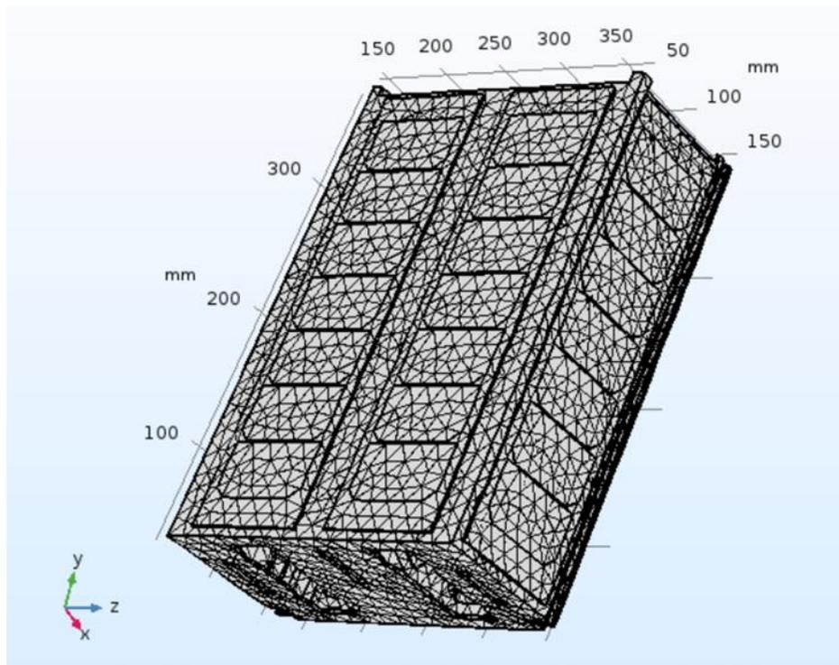
**Figure 46a: Final mesh for Heat Transfer Analysis**
