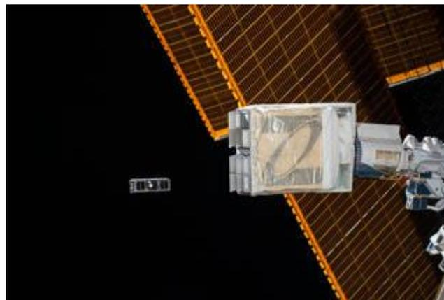
**Figure 3: The NanoRacks CubeSat Deployer (NRCS) 12 on the International Space Station releases ExAlta-1 [12]**
