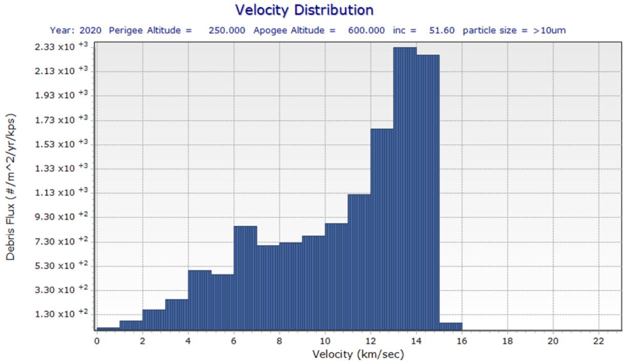
**Figure 43: Velocity distribution of debris**
