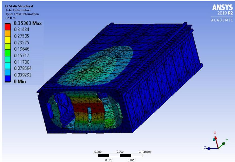
**Figure 39: Structural Load Deformation**
