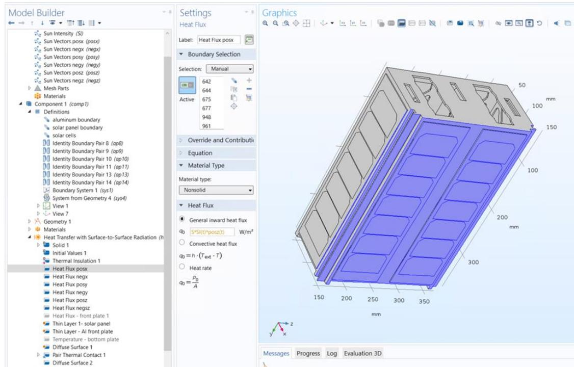
**Figure 48: Heat Flux Definition for Positive X-Face**
