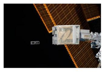
Figure 3: The NanoRacks CubeSat Deployer (NRCSD) 12 on the International Space Station releases ExAlta-1 [12]
