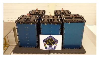
Figure 8: Quadpacks 12U dispenser for Dnepr launch June 2014 [18]
