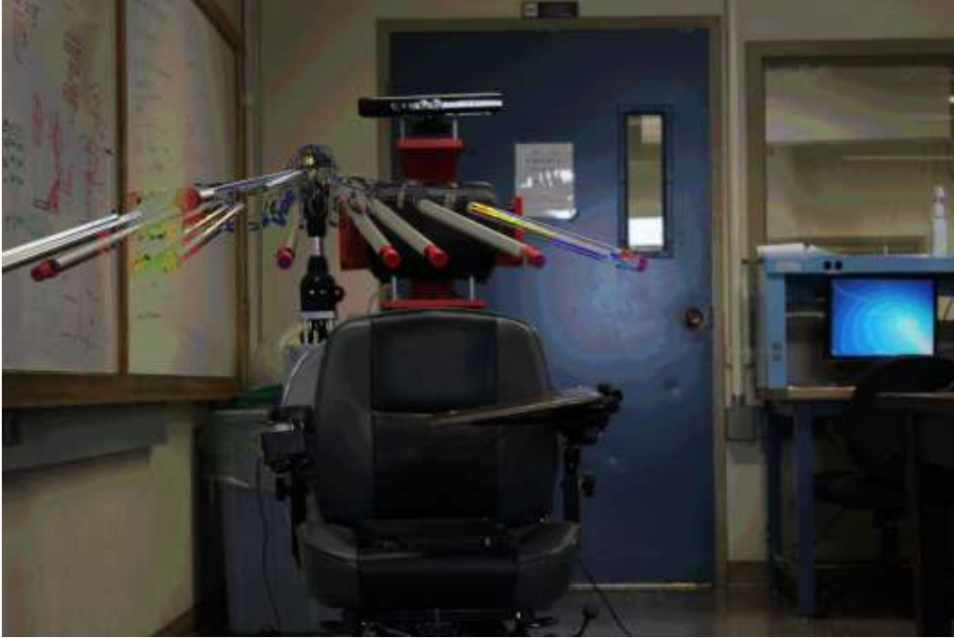
Figure 17: Workspace of Arm – Horizontal
