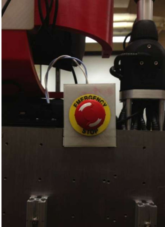
Figure 12: Emergency Stop Button
