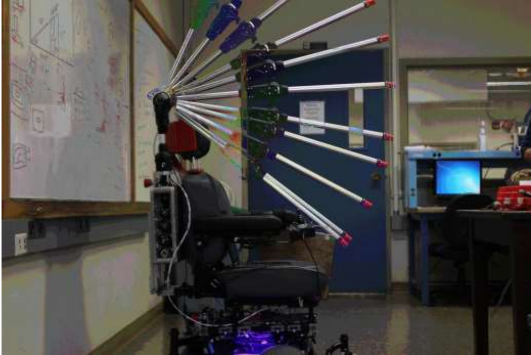
Figure 15: Workspace of Arm – Vertical
