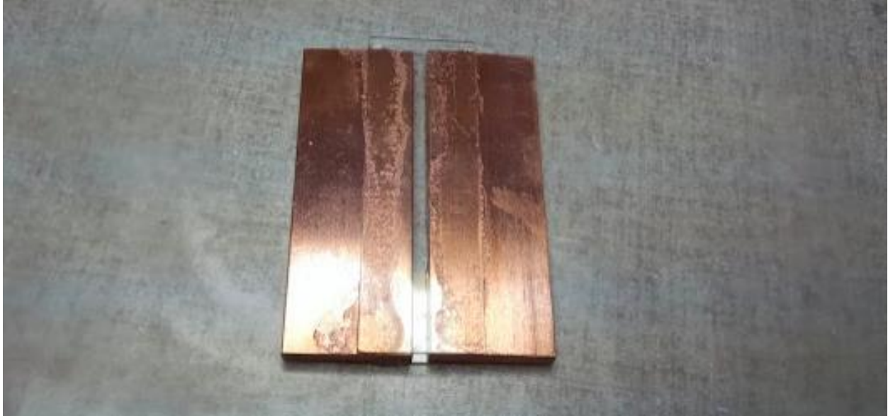
Figure 34: Copper electrodes with glass walls.
