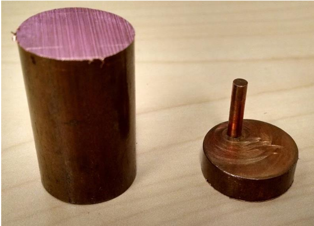
Figure 42: Copper reducing cylinder.
