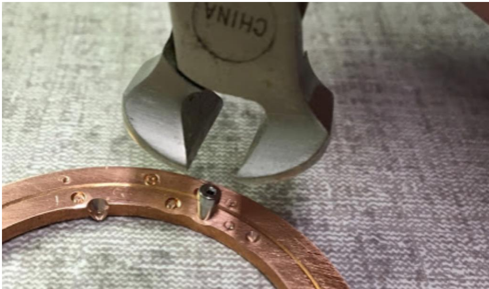
Figure 31: Metal ferrule used to create indentation in copper.
