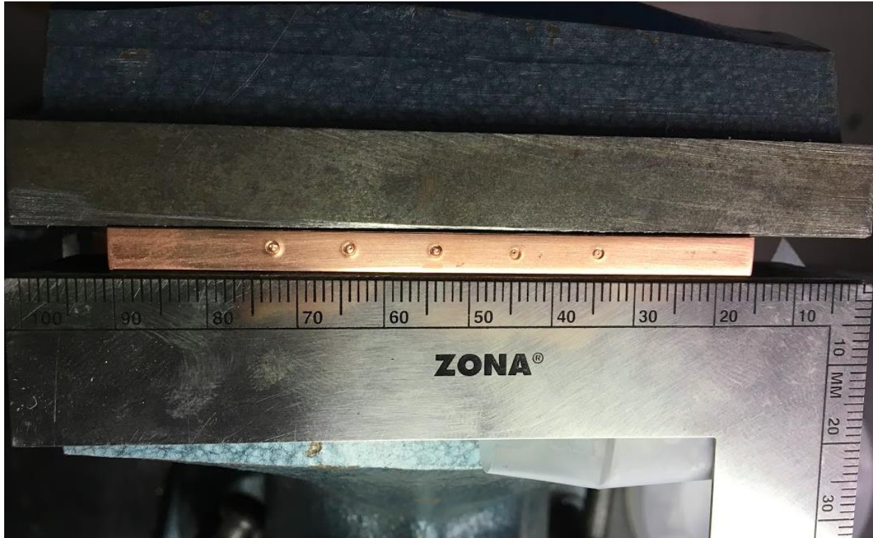
Figure 33: Using the center punch to create nucleation sites in a bench vise. Nucleation sites are numbered sequentially (from channel inlet, left in this image).
