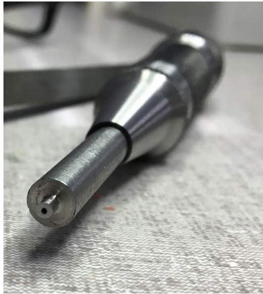
Figure 26: Mechanical Indentation Device
