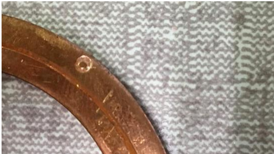
Figure 27: Depression created by designed indentation pin.
