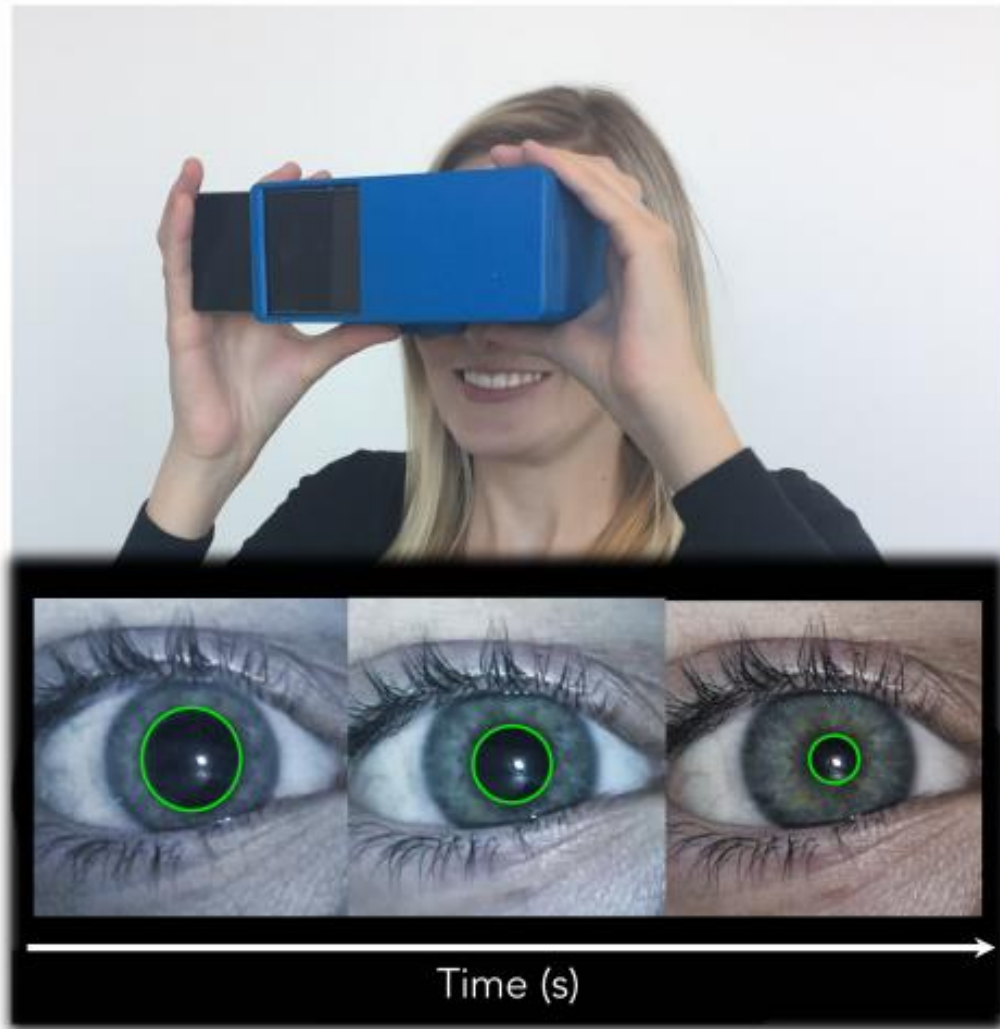
Figure 4: PupilScreen system that measures PLR and lightning that reaches the eye [23]
