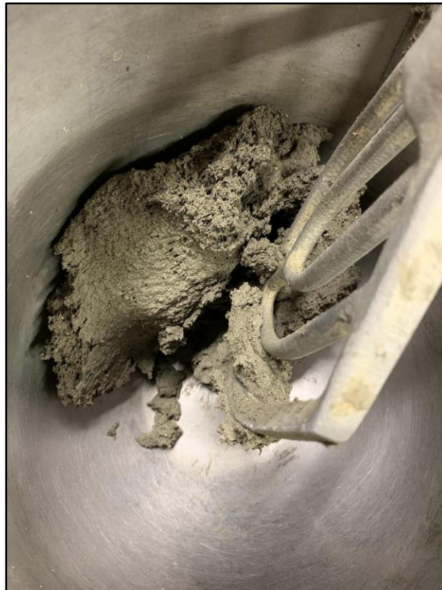
Figure 32: The initial PAM mixture B671SP1.6PAM9.0 clumped together during mixing showing the effects of PAM on the cohesiveness of concrete. At a dose of nine percent by weight of binder, PAM created such a cohesive mix that the concrete was labeled un pumpable.
