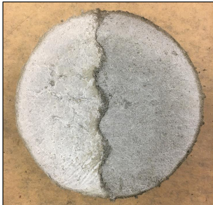
Figure 26: Example of a fully prepared sample for the Brazil disk test with a sinusoidal wave as the interface between the two halves of the concrete disk.
