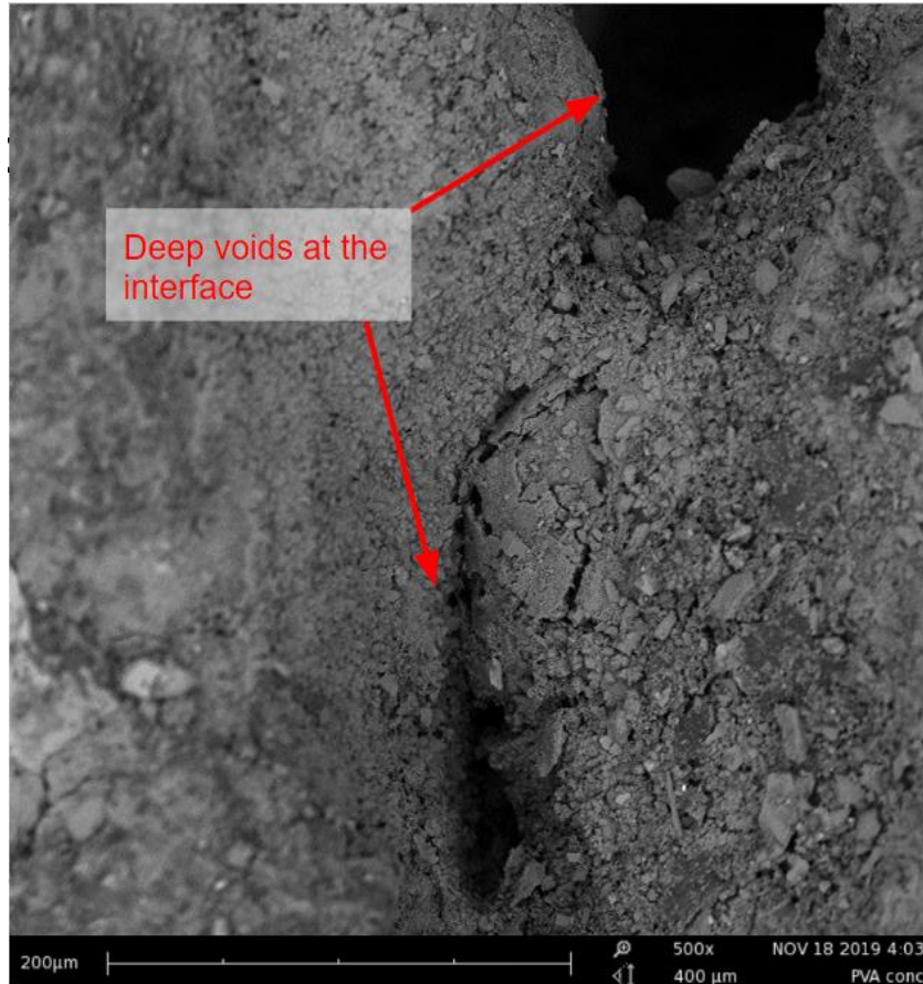
Figure 52: SEM image showing air voids at the PVA interface. These voids are sites for crack propagation along the interface as the tips are locations of stress concentrations.
