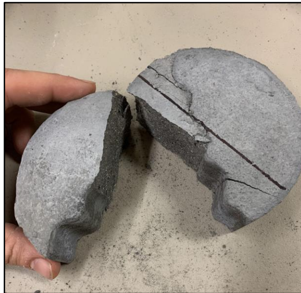
Figure 58: Top view of 3C after breaking at a 25-degree load angle. Within Mode II fracture, sample 3C broke at the highest load of 7,406 lbs. Sample 3C created an essentially homogeneous interface in shear as the sample broke initially in tension through the solid portion of the sample, then sheared once the crack met with the interface.
