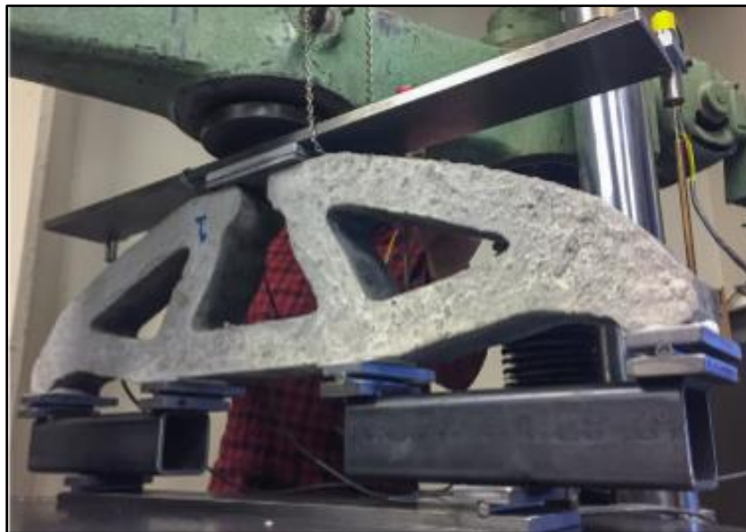
Figure 1: Example of a topology optimized beam design taken from “Topology-optimized design, construction and experimental evaluation of concrete beams” (Jewett & Carstensen, 2019).
