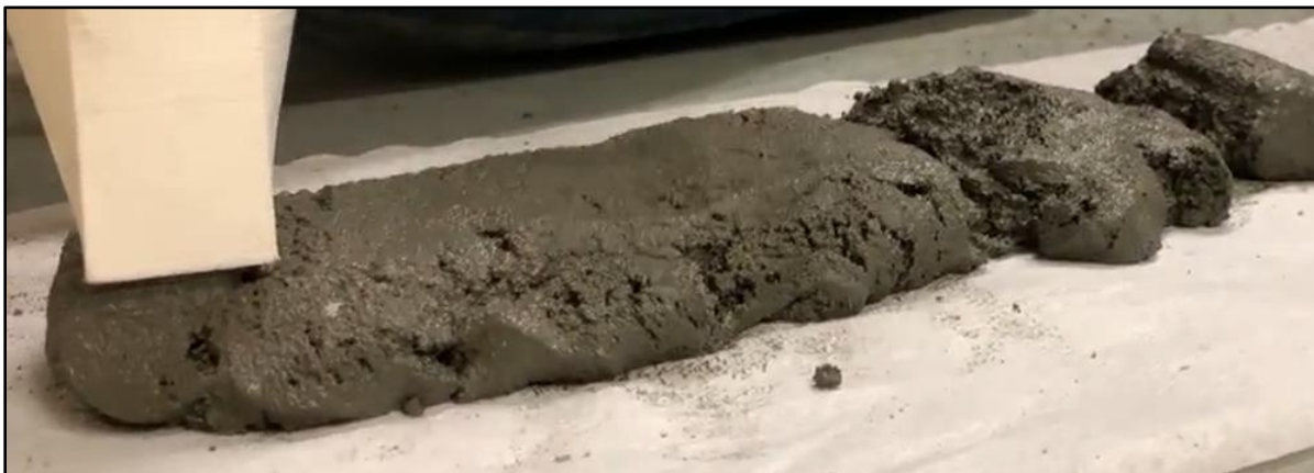
Figure 36: Filament for mix design B690SP1.2PVA0.25 illustrating the deformed filament shape. The surface quality of the layers for the mix designs ranked fourth and fifth showed breaks and uneven thicknesses. There was a clear lack of layer cohesion and shape retention for these mix designs.
