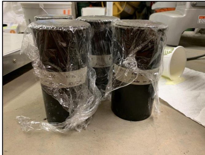
Figure 21: Molds filled with wet concrete to be cured for the compression test.
