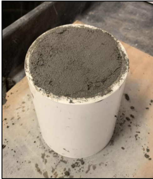
Figure 15: 101.6 mm x 101.6 mm Ø cylinder for estimating the pumpability and assessing consistency of trial mixtures.
