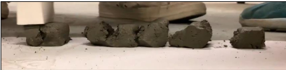
Figure 35: Extrusion of base mix design, B508SF, illustrates the discontinuous filaments seen in the mixes ranked first through third. These mixes were difficult to pump and lacked cohesion.
