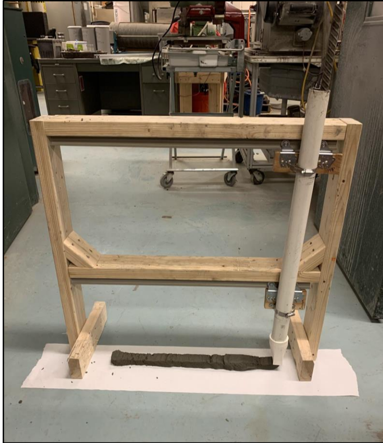
Figure 19: Hand extrusion prototype used for extrudability testing consisting of a PVC pipe and 3D printed nozzle fastened to rollers on a wooden frame. Mix designs were ranked based on the consistency of the mix's flow during extrusion, the amount of excess water, the surface finish of the filament, and its deformation after extrusion.
