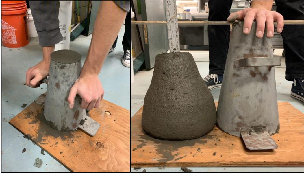
Figure 18: Standard slump cone complying to ASTM C143 used to assess pumpability.
