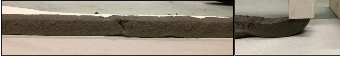
Figure 37: (Left) Extruded filament for PAM mix B571.2SP1.6PAM0.9. (Right) PAM mix B571.2SP1.6PAM0.9 being extruded from the nozzle. This mix retained its shape without noticeable deformation and produced a continuous layer. Any inconsistencies can be attributed to human error during extrusion.
