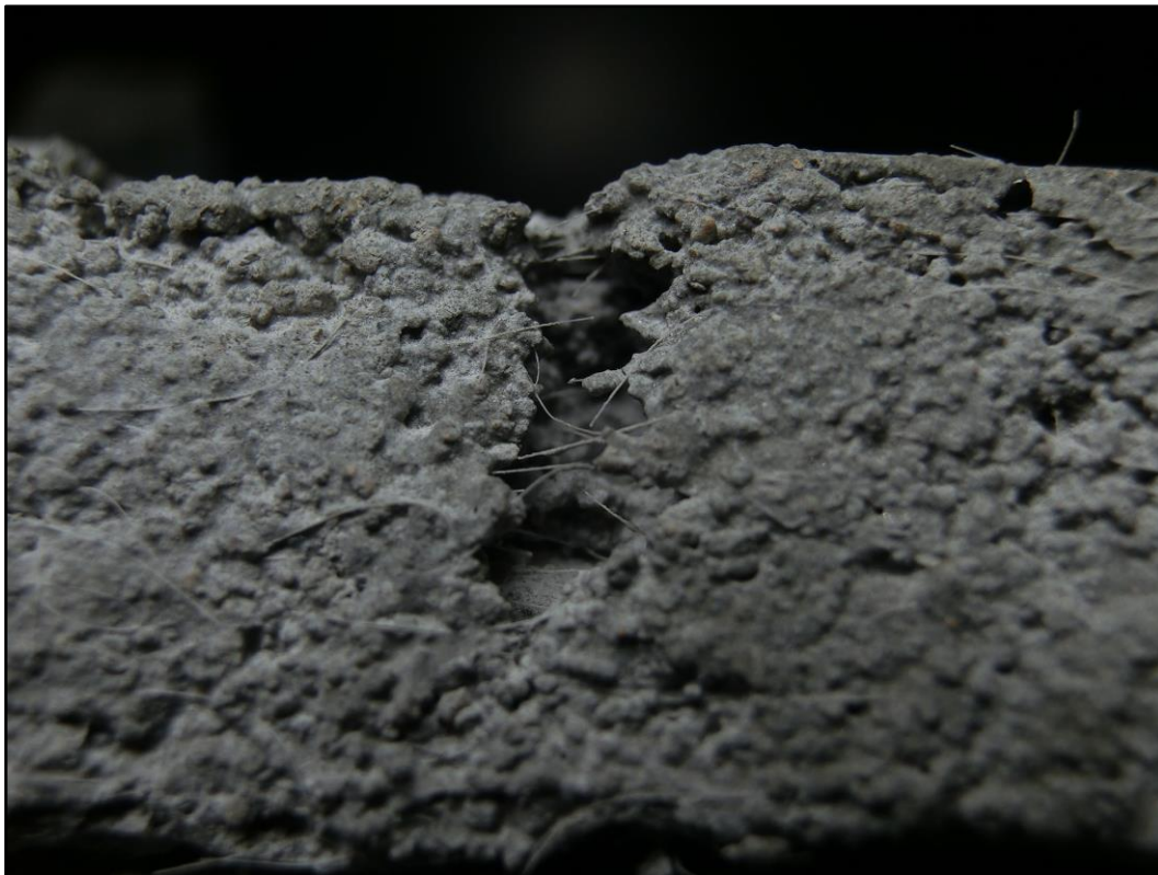
Figure 48: Macroscopic image of the surface of a printed layer showing fibers at the layer surface oriented longitudinally along the length of the layer.
