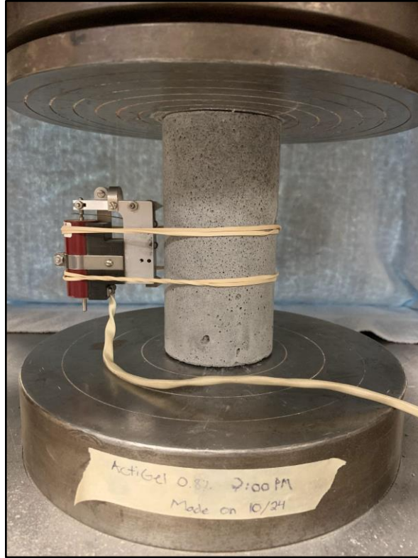
Figure 23: Test setup for compression testing including an extensometer to record strain values for the sample.
