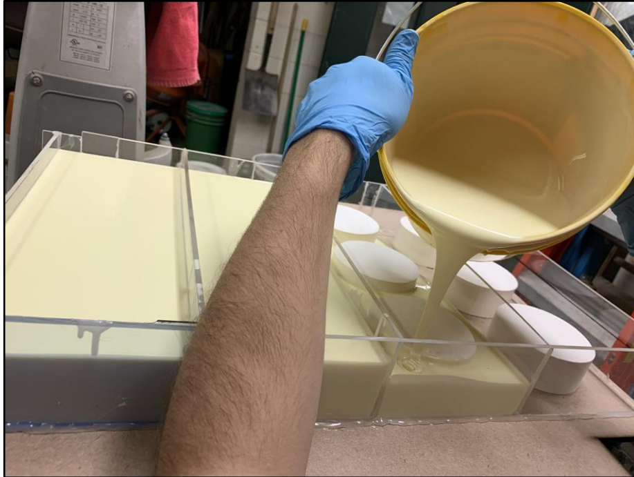
Figure 28: Pouring silicone rubber into forms to make molds for Brazilian disk samples.
