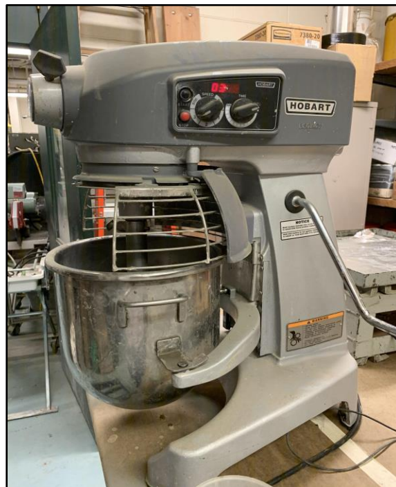
Figure 14: Hobart Legacy 120 Mixer used to maintain a consistent mixing speed in each step of the mixing procedure.
