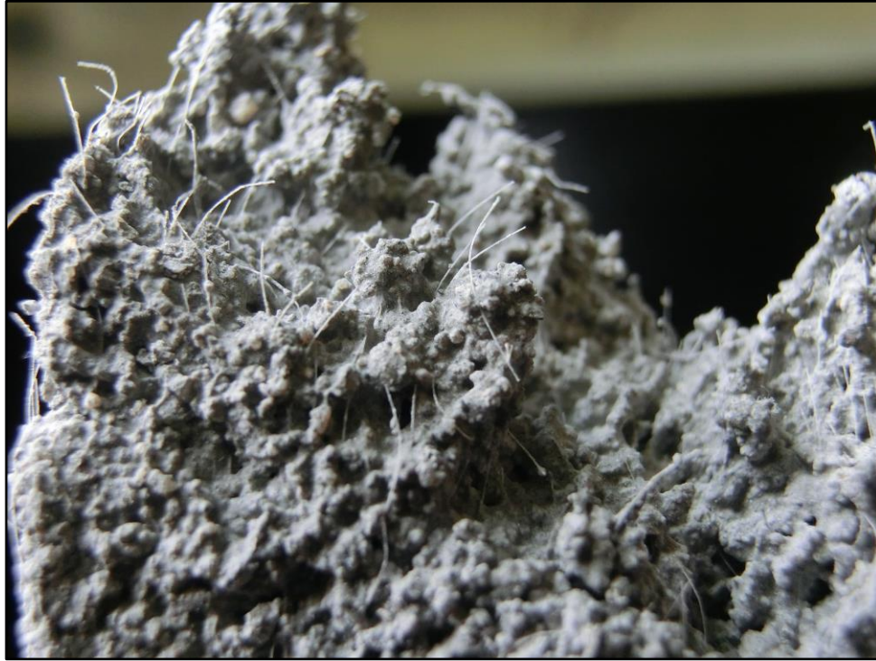
Figure 49: Macroscopic image of the end of a printed layer showing interior fibers also orientated longitudinally along the length of the layer. This consistent fiber orientation could result in reduced shrinkage and cracking resistance perpendicular to the length of the layer.
