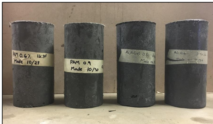
Figure 22: Fully cured cylinders ready for compression testing.
