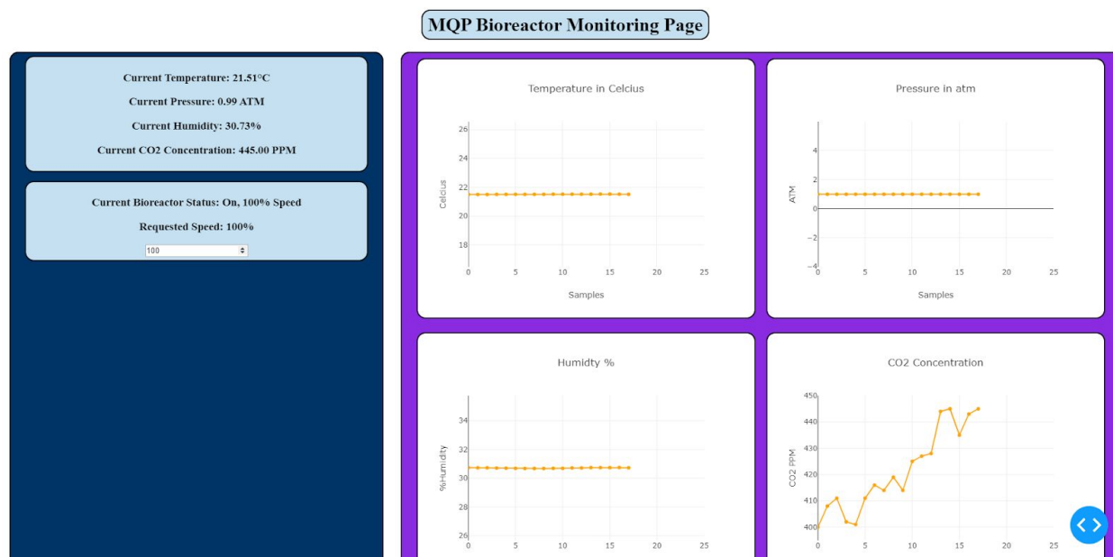
Figure 6.3: Bioreactor monitoring and controlling webpage
