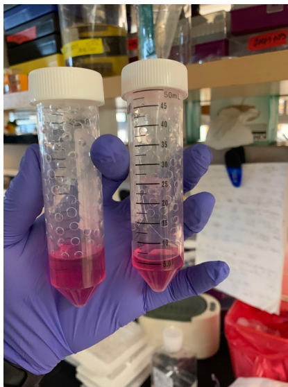
Figure 5.5: Note about 4mL of media was lost in one tube over the two day incubation period
