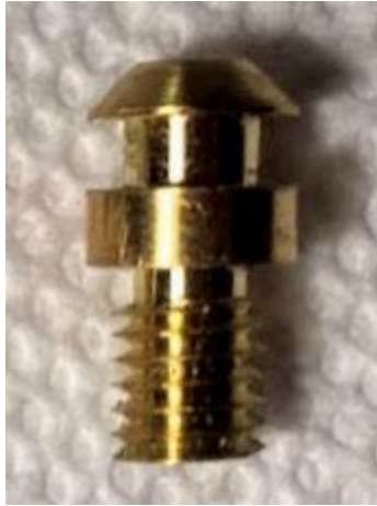
Figure 8: Manufactured Product of the Solenoid Print Nozzle
