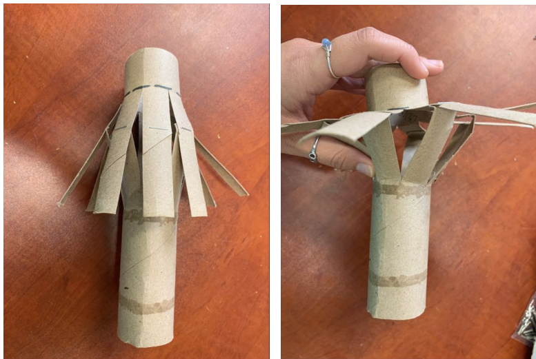
Figure 14: Cardboard Constructed Prototype of Ratcheting System
