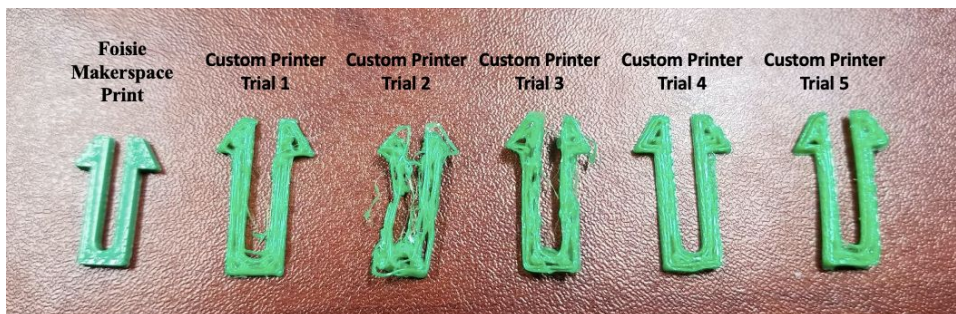
Figure 21: Compared Results of Various Print Settings Used for the Actuator Buckle
