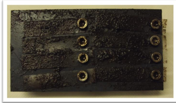
6.1.1.3.3 Image of the Plastic Films on the Plate in the Bottom of the Reactor
